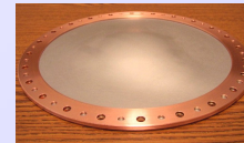
An 8-cm-radius curved Be window made by Brush-Wellman for 805-MHz RF cavity tests. An equivalent 21-cm-radius window will be used for the MICE 201-MHz cavity.
