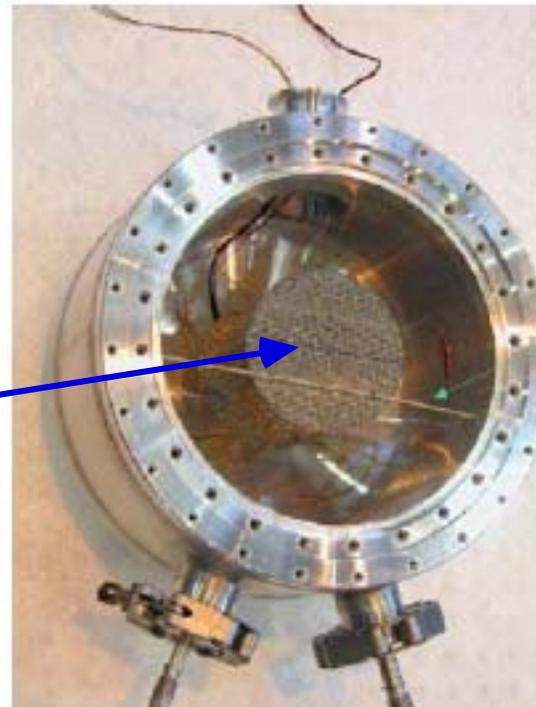
Array of heating wires
