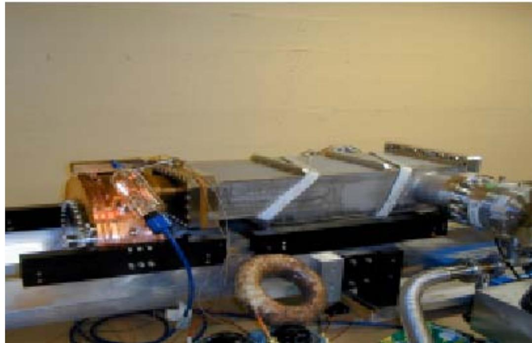
Closed-cell 805-MHz prototype undergoing bake-out at LBL (now under high-power test in Lab G)
