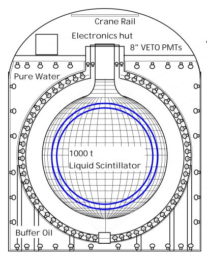
Anti 20" PMTs Kevlar Suspension Rope Tyvek Sheet/ 18m Stainless Tank 17"/20" inner PMTs Rock Wall/ PE sheet/ Radon Blocking Resin/ Tyvek reflector **PET Black Sheet** EVOH/3Nylon/EVOH 13m Balloon Acrylic Sphere (3mm t) Fiducial Volume for Reactor Neutrinos (600t) Fiducial Volume for
