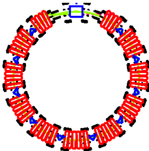
Figure 6. Schematic diagram of cooling ring based on tilted solenoids. The wedge absorbers (small triangles) are located between the RF cavities and solenoids. Injection and extraction take place at the top of the diagram.
