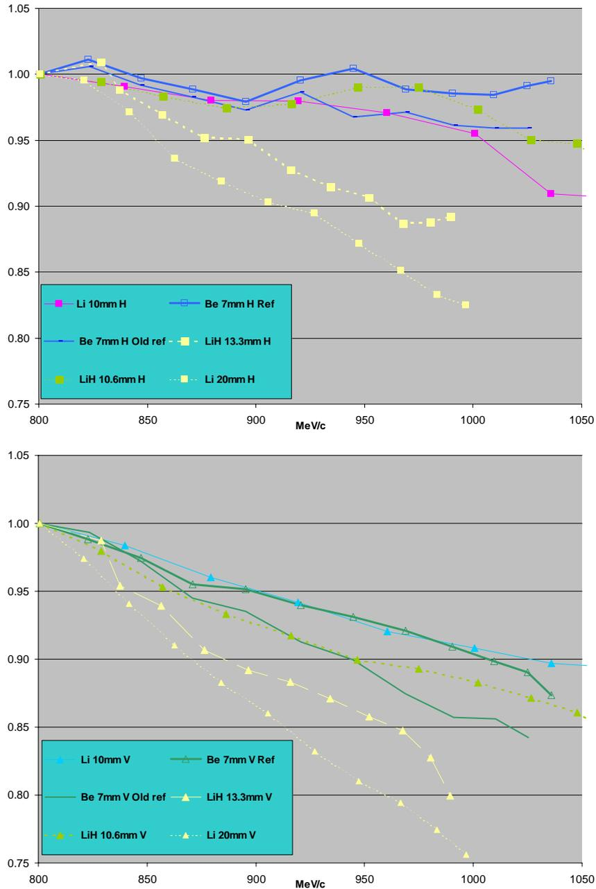
Fig. 1. Results of the tracking with ACCSIM [2] of initial annuli in phase space of  $4000 \pi$  mm mrad, corresponding to an r.m.s. emittance of  $2000 \pi$  mm mrad (physical) or  $15000 \pi$  mm mrad (normalized). Show is the cooling factor of normalised rms emittances in the horizontal (top) and vertical (bottom) plane w.r.t. the initial value at 800 MeV/c.
