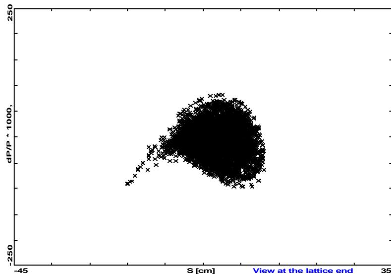
Longitudinal phase space at the beginning and at the end of Linear Pre-accelerator
