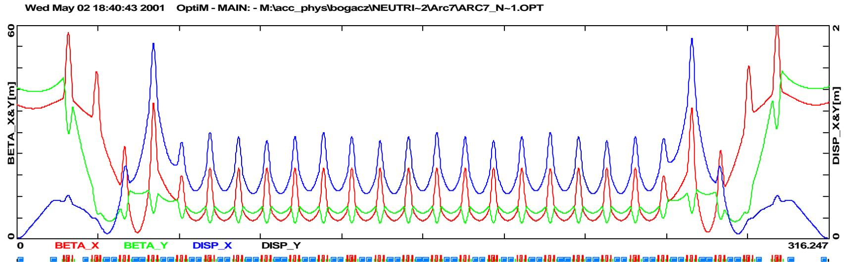
❖ Optimized linac optics for multi pass beams – smooth transition Arc-linac
