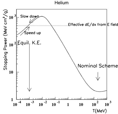
**Figure 1.**  $dE/dx$  in Helium as a function of kinetic energy,  $T$ , for  $\mu^+$ . The effective  $dE/dx$  resulting from an external electric field is superimposed. An equilibrium kinetic energy near 1 KeV would result. The nominal scheme discussed for a Neutrino Factory would cool muons near  $T=200$  MeV.
