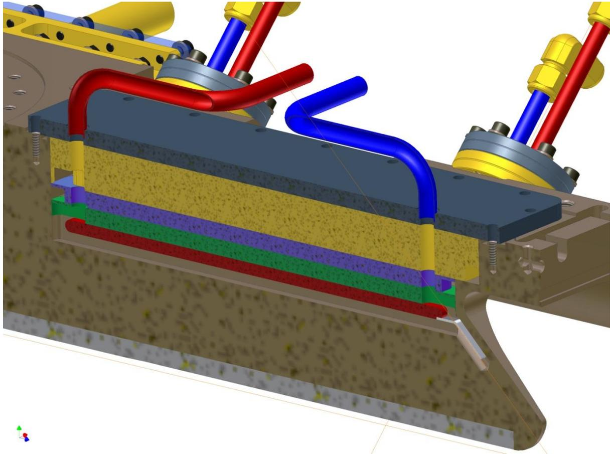
Figure 32: Section view showing major vane fitted with cooling baffles
