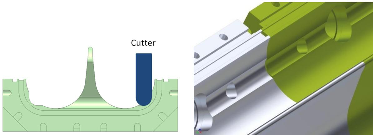
**Figure 43: Diameter 25mm ball nosed cutter used to create modulation compensation grooves**
