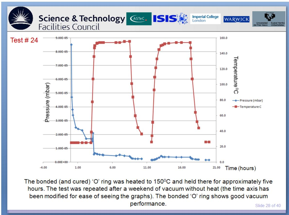
Figure 21: Vacuum performance of 3D O ring at elevated temperatures (talk # 64)
