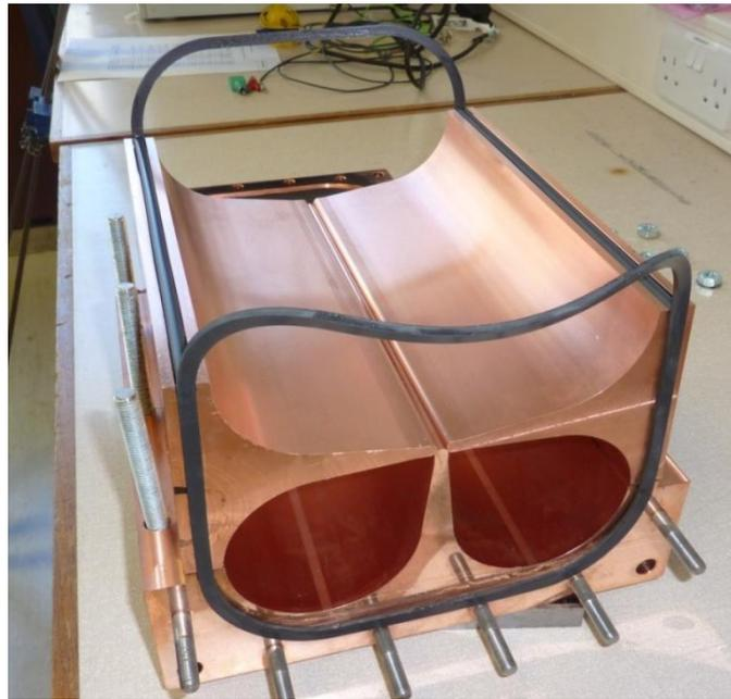
Figure 20: Weld test model with 3D rubber seal in place
