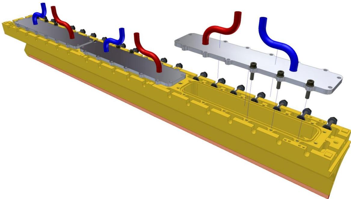
Figure 34: Minor vane cooling channel lids – baffles not shown
