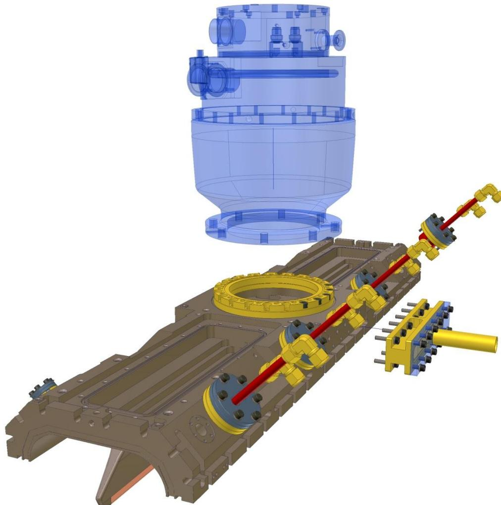
Figure 17: Exploded view of major vane showing vacuum pump mounting
