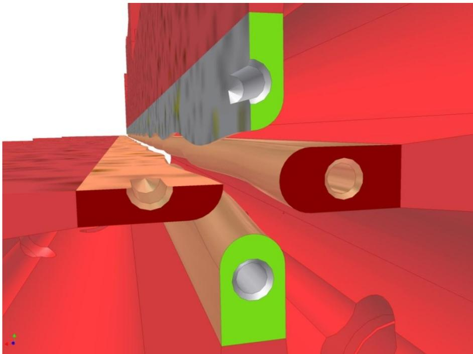
Figure 6: Close-up view showing the vane tip modulations that produce the longitudinal electric field.
