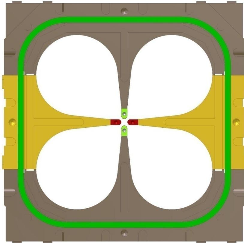
Figure 4: End view of RFQ section 1
