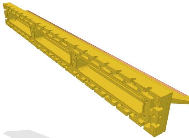
Figure 11: RFQ minor vane – showing external features
