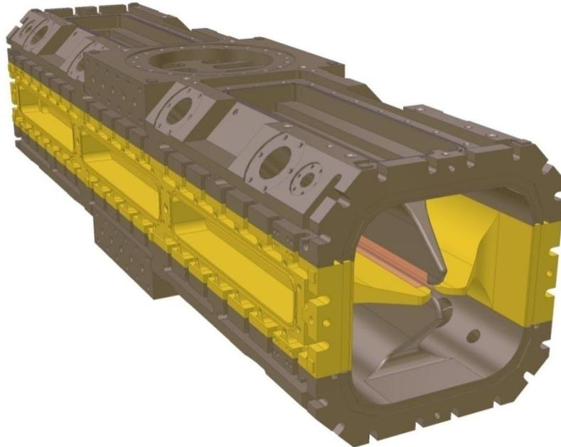
**Figure 1: One metre long RFQ – an assembly of two pairs of parts**
