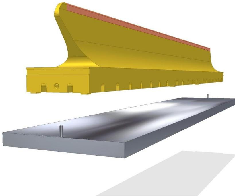
Figure 14: Minor vane with machining mounting plate
