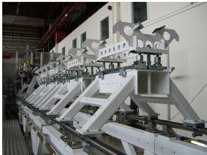
**Figure 36: Four RFQ support frames on the FETS**
