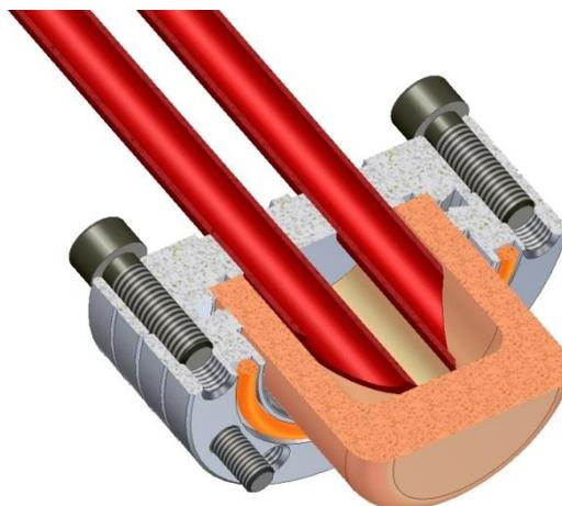
**Figure 28: Section view of static tuner**
