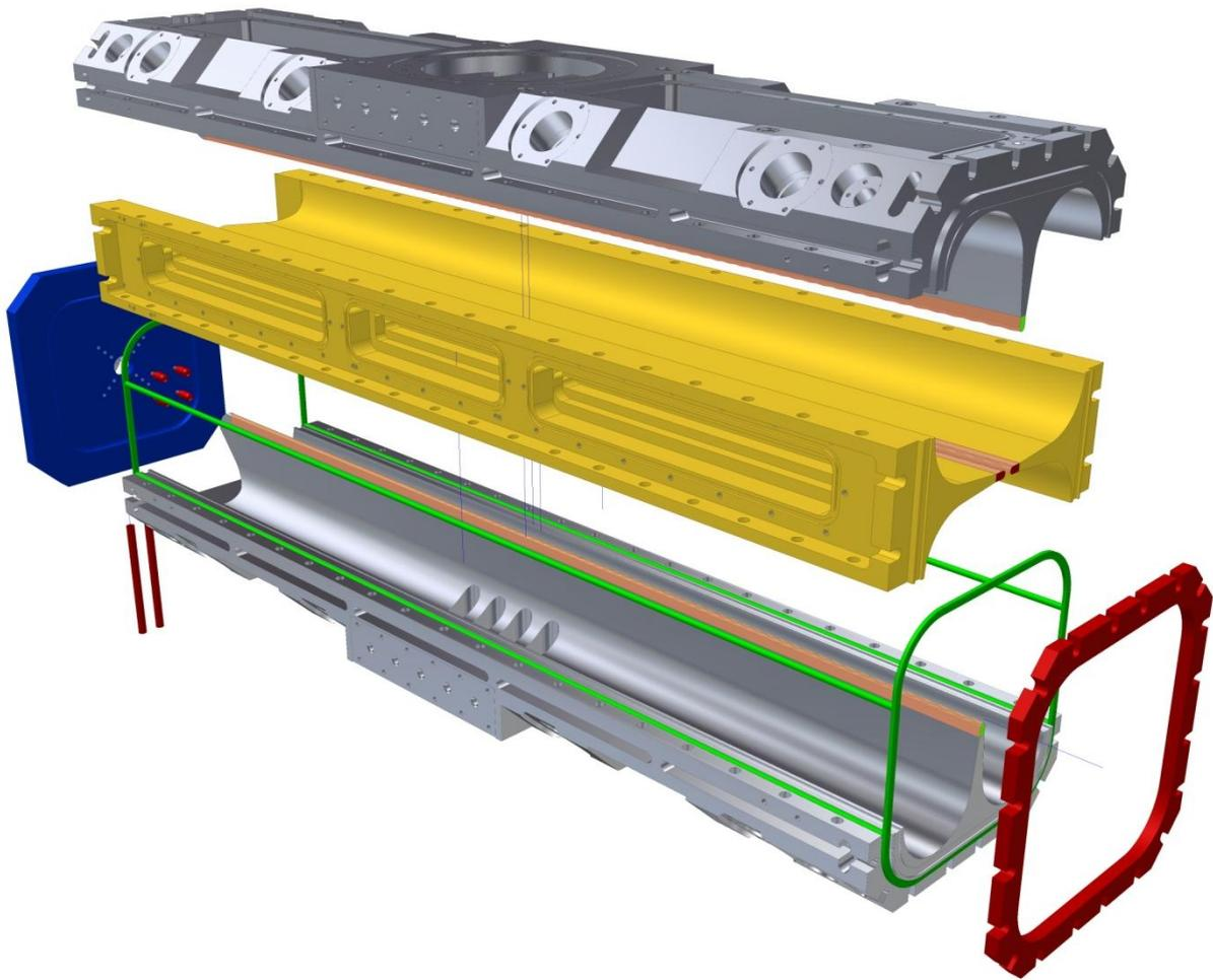
Figure 22: Exploded view showing 3D O ring vacuum seal
