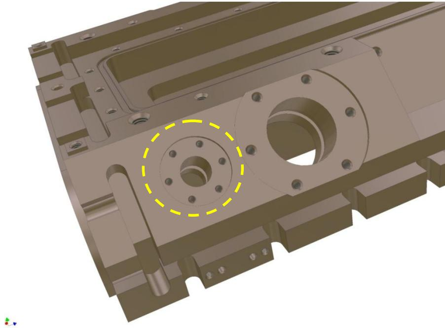
Figure 24: Probe Port location on RFQ major vane
