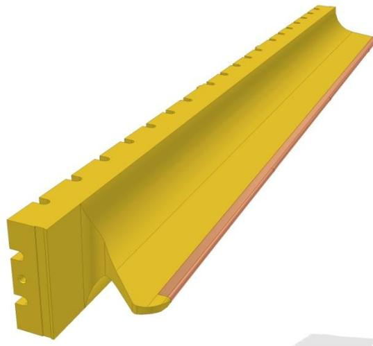
Figure 12: RFQ minor vane – showing internal vane
