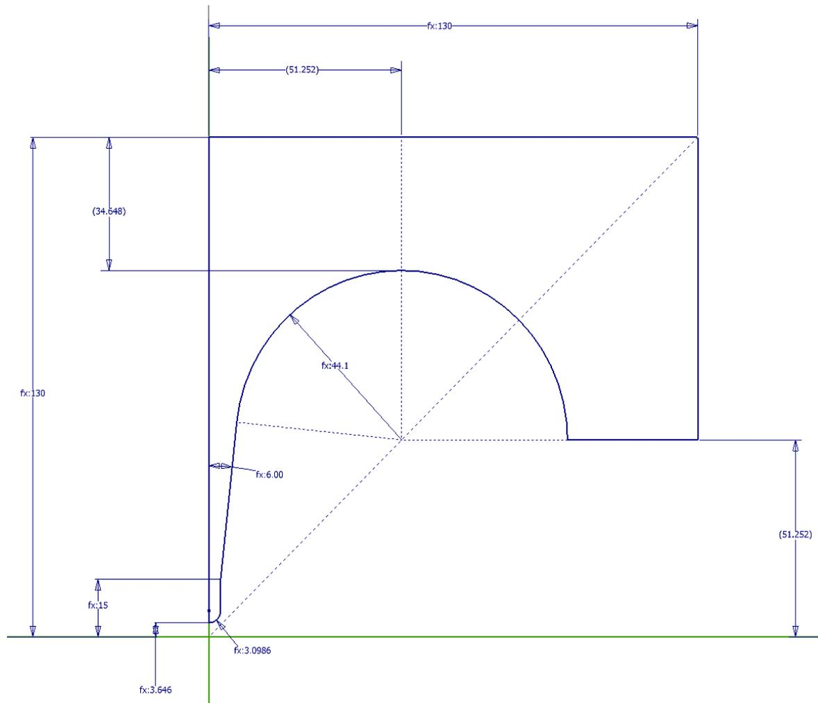
**Figure 3: 2D sketch that controls the geometry of the major and minor vanes**
