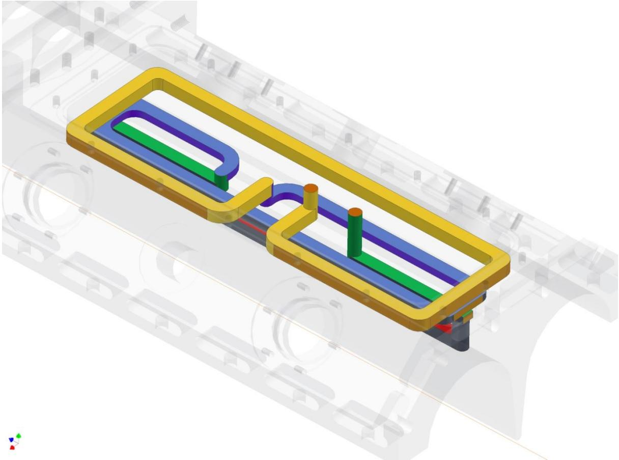
Figure 33: Coolant path around baffles in major vane
