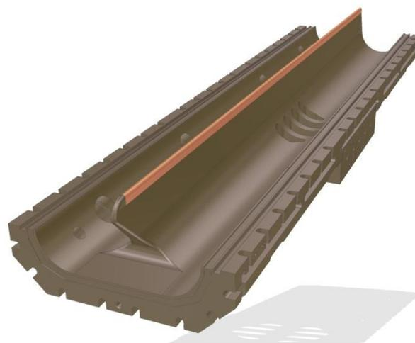
Figure 10: RFQ major vane – showing internal features
