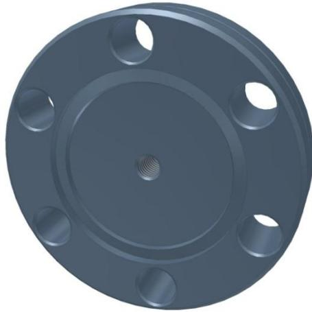
**Figure 26: Probe port modified CF16 blank flange**
