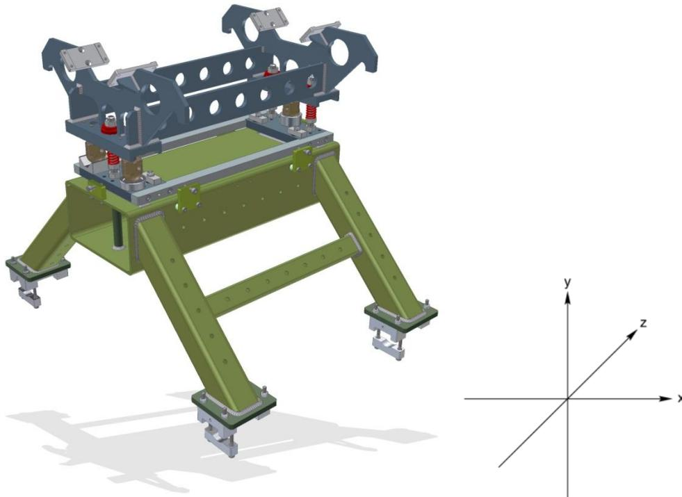
**Figure 35: RFQ 1m section support system**
