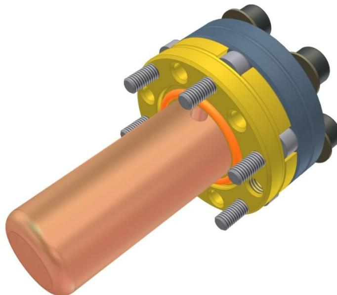
Figure 23: Probe Port plug assembly
