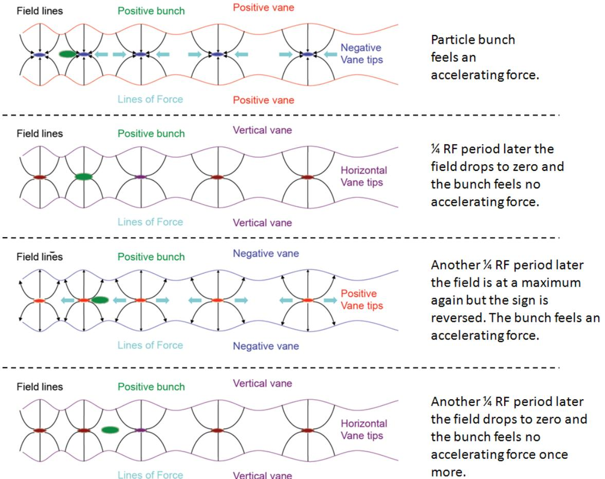
**Figure 7:** Sequence to show how the vane modulations accelerate a particle bunch – Simon Jolly
