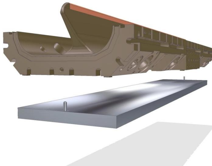
**Figure 13: Major vane with machining mounting plate**
