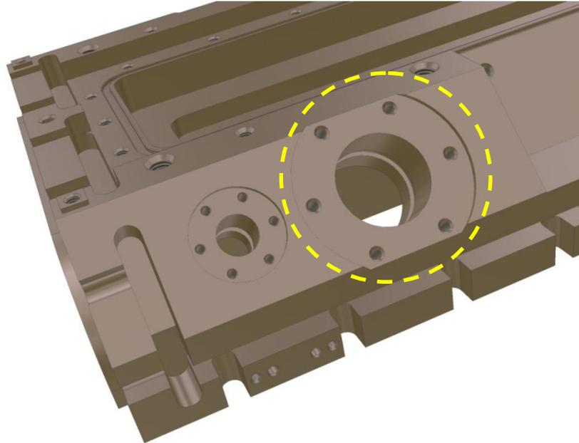
**Figure 27: Tuner port location on RFQ major vane**
