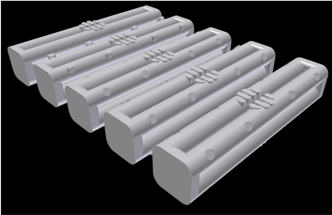
**Figure 15: 3D CAD data in SAT format used to study the effect of tuner depth on frequency**
