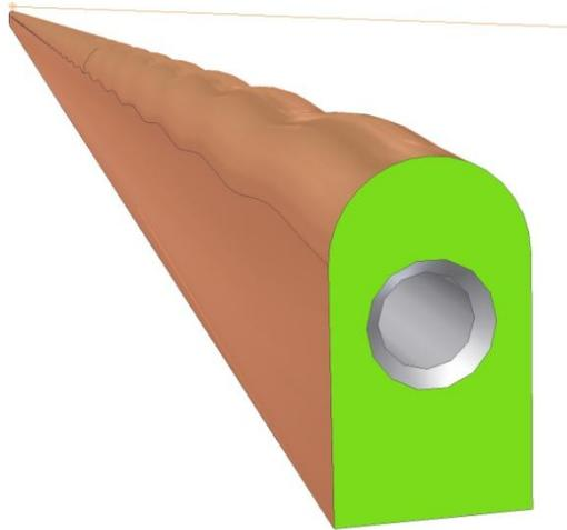
**Figure 8: A vane tip with modulations**
