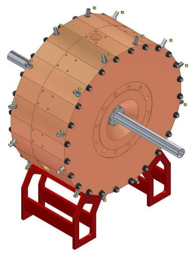
This design is based upon a CERN design. It is a thick walled structure made in two 'halves' that are bolted together. The RF seal is Helicoflex. Cooling channels run through the thick walls. The beam pipe shown here is a 30mm ID welded to a DN40CF flange. The total length (in Z) is 50mm + the inside length, in this case it is 250mm.
