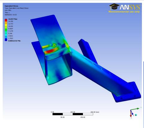
Maximum equivalent stress = 16MPa Maximum deformation = 0.04 mm
