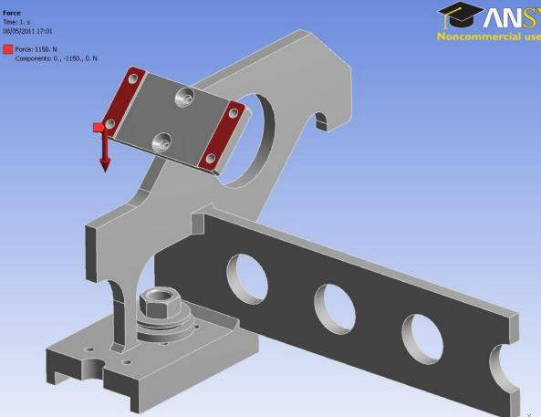
QN: What is the stress and deformation in the RFQ support cradle due to the weight of the RFQ and the ancillary components?
