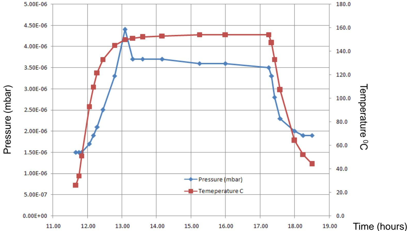
Showing just the second heating cycle for Test# 24. During the high temperature phase the pressure initially rose and then began to fall as the out-gassing decreased. Finally the pressure began to fall rapidly with falling temperature.
