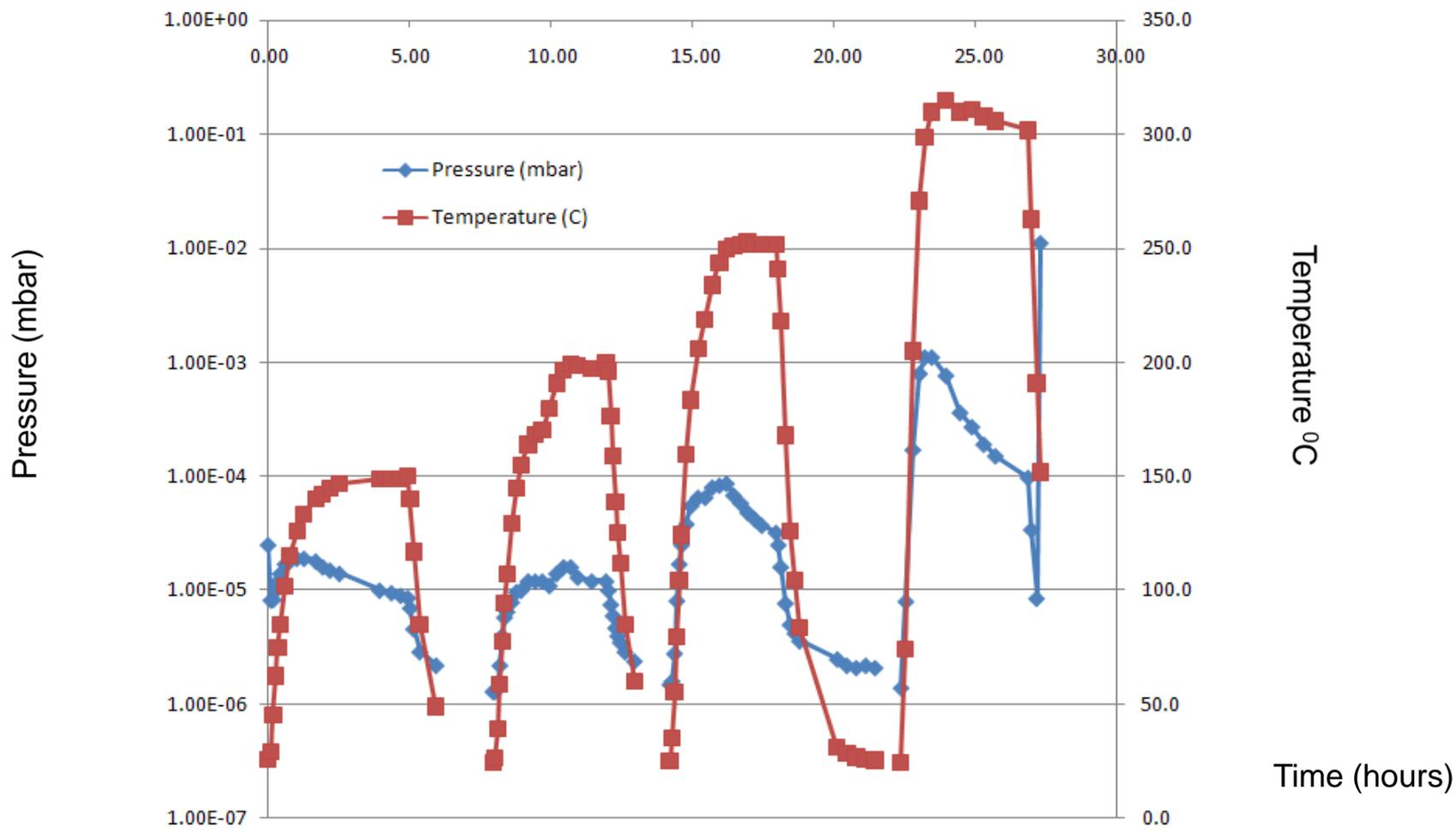
Results shown consecutively for tests 26 through to 29 which correspond to temperatures of 150°C, 200°C, 250°C and 300°C.
