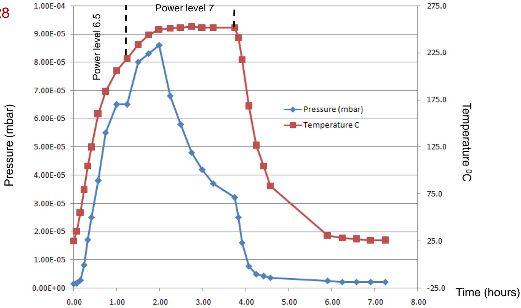
A repeat of test 26 but this time taking the system up to 250°C and holding.
