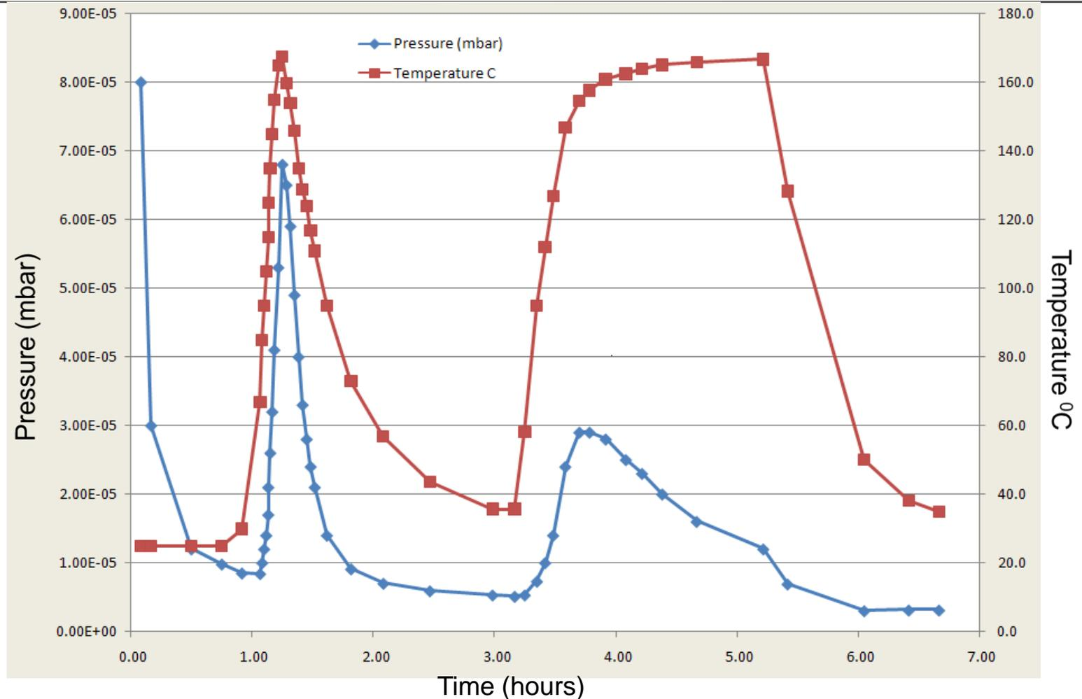
The 'O' ring was heated to 150°C and then immediately cooled followed by heating again to 150°C and holding there for two hours. During the high temperature period the pressure initially rose and then began to fall as expected. This test is the benchmark for tests 24 and 25.
