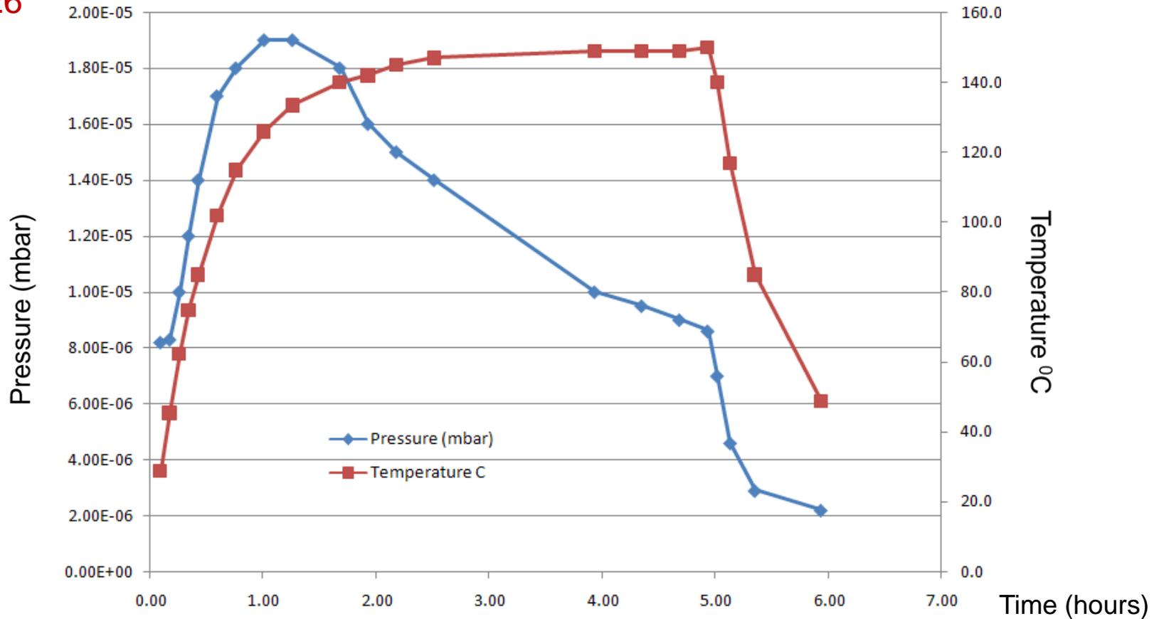
The 'O' ring flanges were heated to 150°C and held at that temperature for approximately 3 hours.
