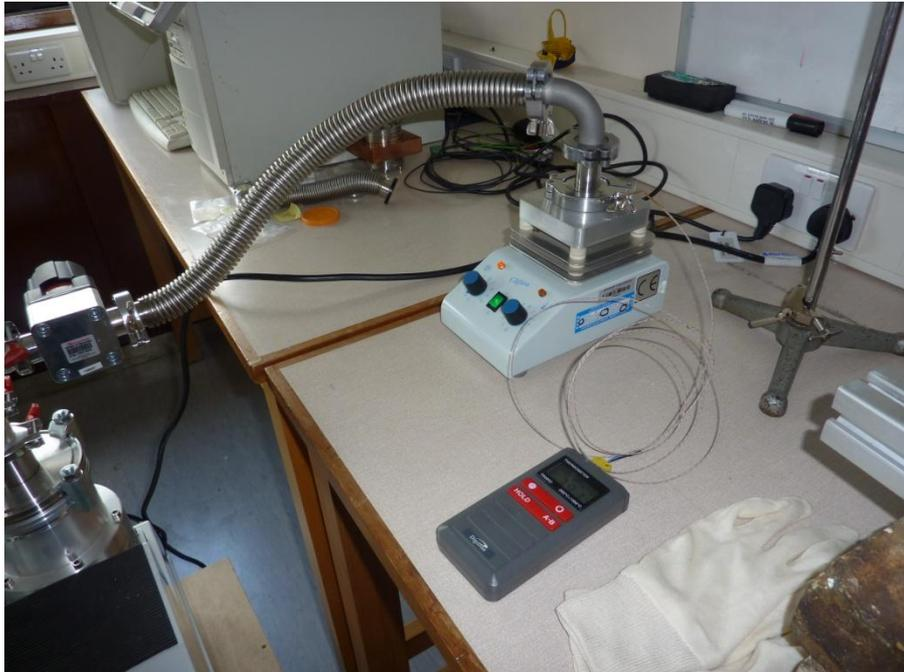
The heater set to power level 4 will take the 'O' ring under test to just over 150°C.
