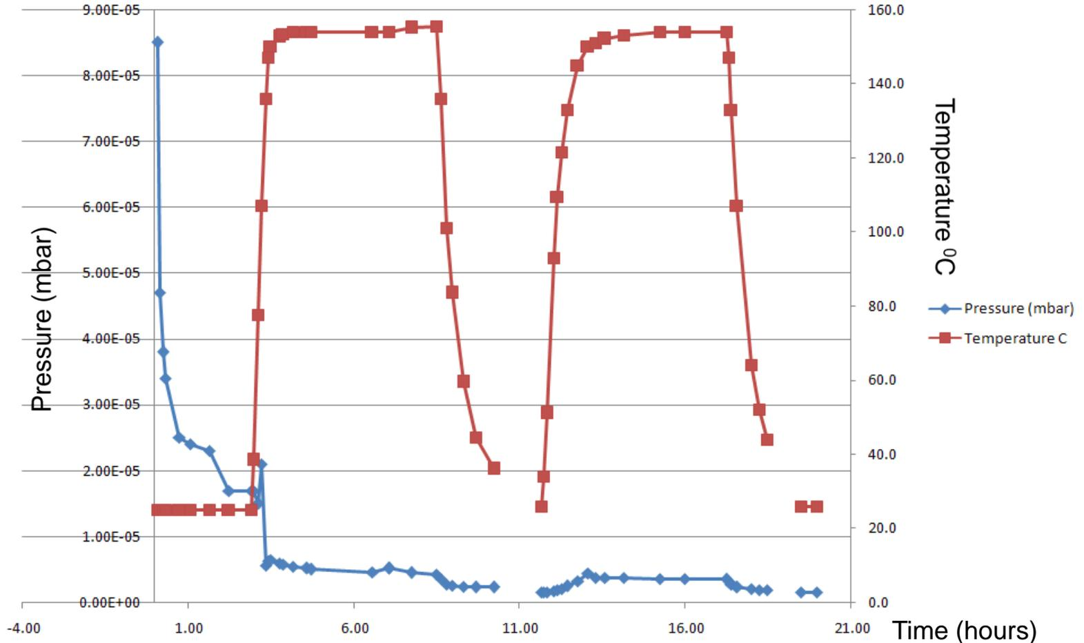
The bonded (and cured) 'O' ring was heated to 150°C and held there for approximately five hours. The test was repeated after a weekend of vacuum without heat (the time axis has been modified for ease of seeing the graphs). The bonded 'O' ring shows good vacuum performance.
