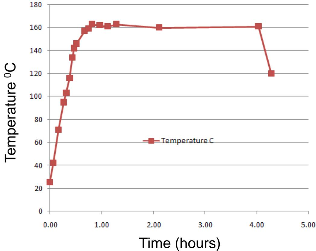
Adhesive cure cycle for the 'O' ring to be used in Test # 24.
