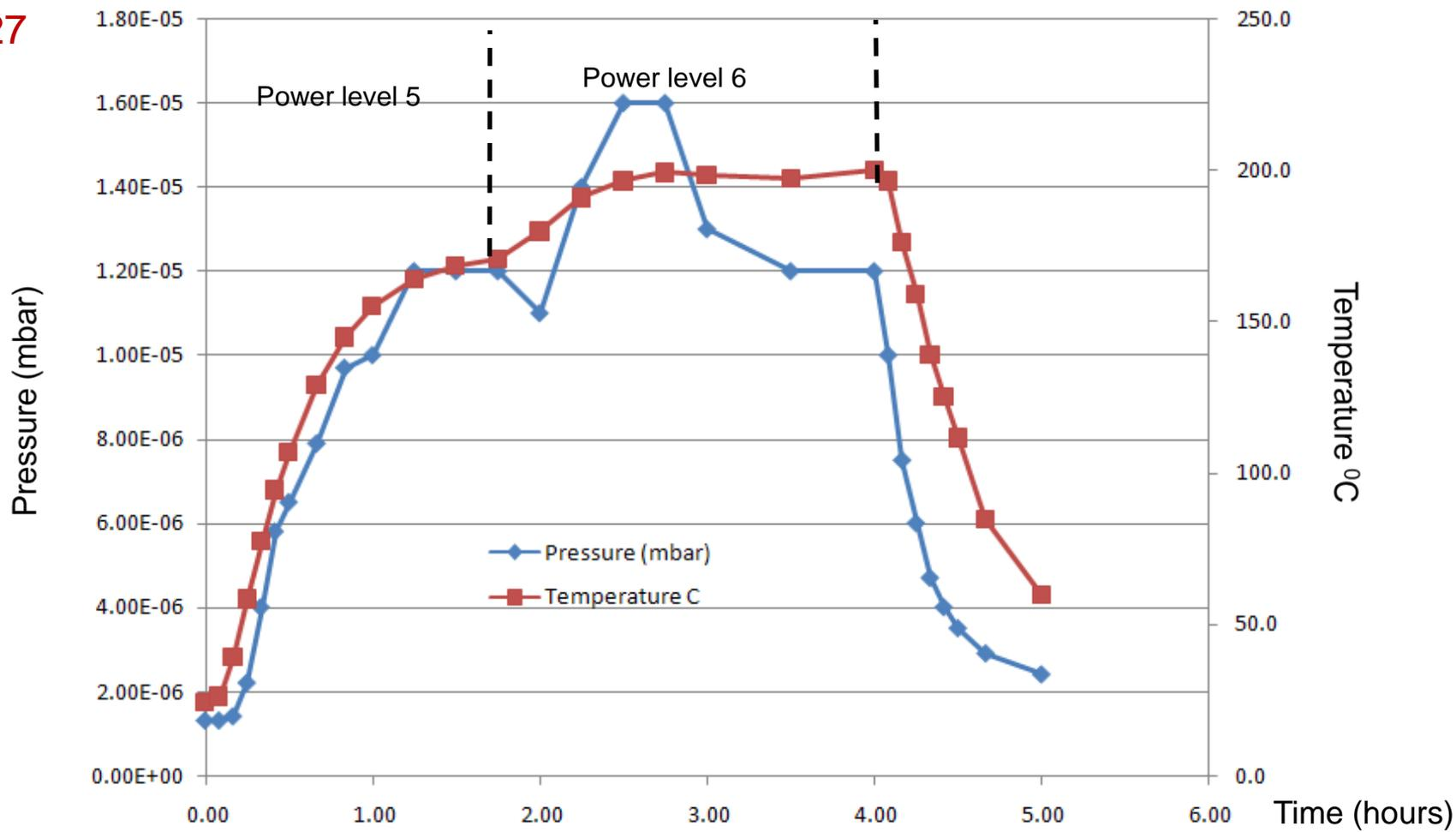
A repeat of test 26 but this time taking the system up to 200°C and holding.
