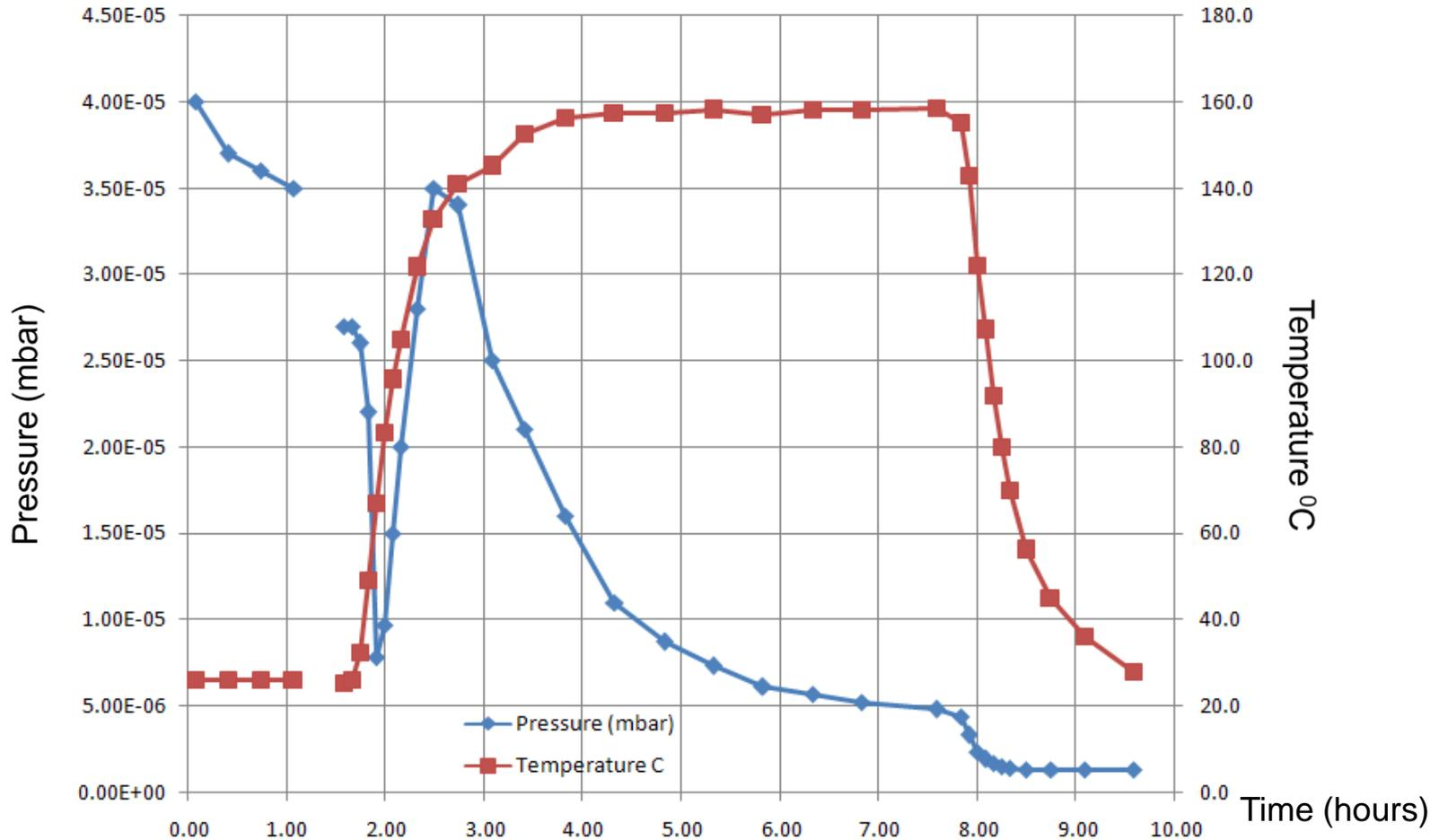
The 'O' ring will have been cured in place by the thermal cycle. The vacuum performance appears to be consistent with that of the cured O ring (test # 24) and that of the complete O ring (test # 23). I cannot explain the sudden pressure drop during the heating up phase. Note that the initial pumping at 0 to 1 hour was in reality 15 hours prior to the heating cycle.
