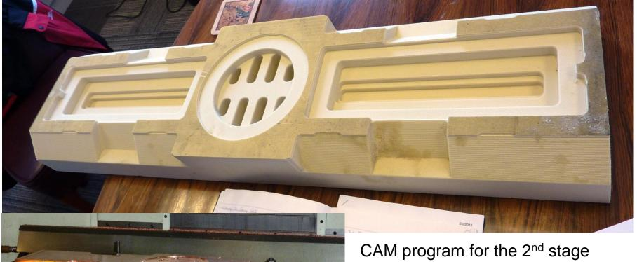
roughing (+2mm) proved in foam model (4 hr operation). Errors are rare but when the material value is high it is worth checking. The next stage is to re-produce this in copper (12 hr operation).
