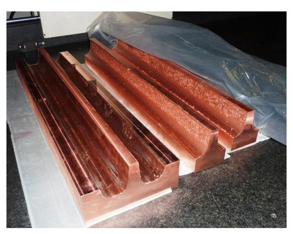
All four blocks for RFQ section 1 have been rough machined to +10mm on the vane side. The largest deflection seen so far is 0.18mm.
