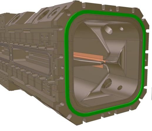
Assume that the RFQ is assembled to its dowelled position with the 3D O ring in place.
