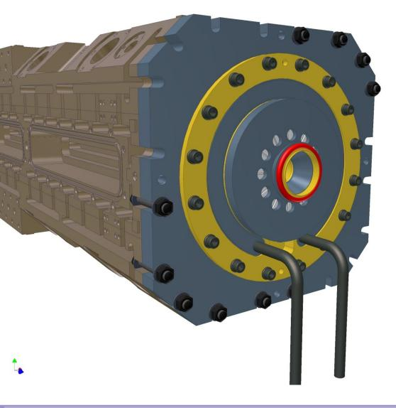
The KF40 O ring seal is added.
