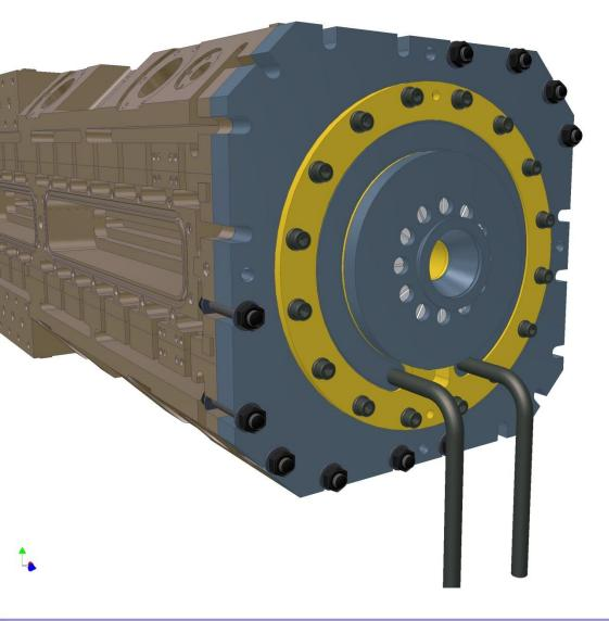
Because the cover is secured using Nylon screws! The screws must be electrically non-conductive to avoid short cutting the current path.
