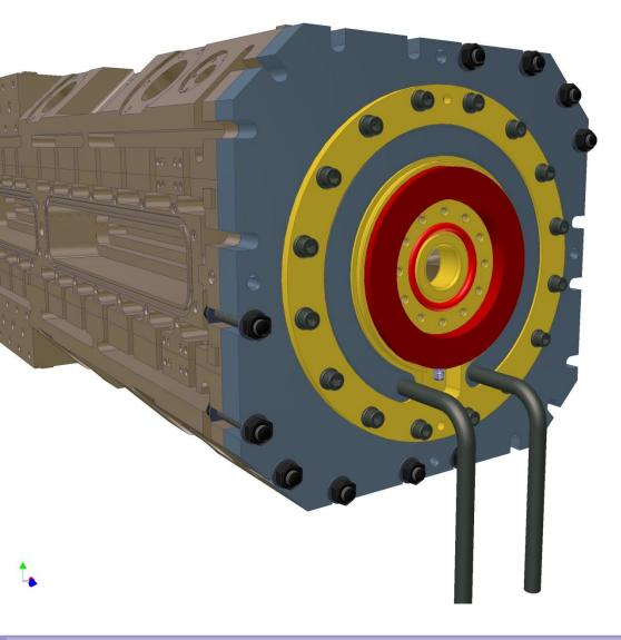
And the vacuum seal is placed in its groove.
