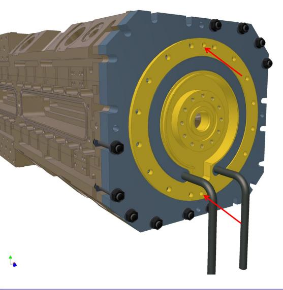
The pre-brazed copper insert assembly has its O ring vacuum seal and copper fingers added.
