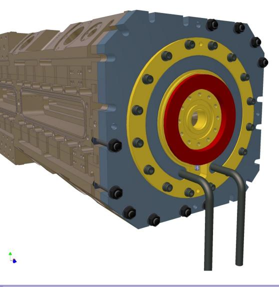
The toroid is placed into its pocket.
