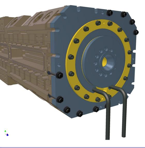
And now the stainless steel toroid cover can be added and tightened until the faces meet. Note that the cover locates on a small lip (arrowed) so that it distributes the vertical load due to the weight of the VAT valve.
