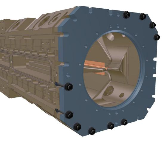
The end flange can now be bolted up tight until the faces meet.
