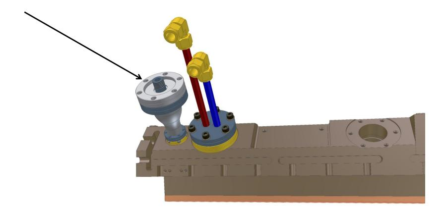
The loop can be rotated by undoing the 6 x M6 screws (not shown) arrowed and rotating the flange centre piece.
