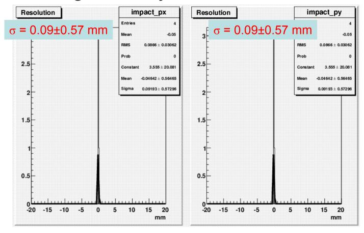
Too small: single chamber resolution should be ~200um. Smaller impact than for DESY (40 Gev instead of 4 GeV) Open to suggestion on how to calculate the resolution (fit?)
