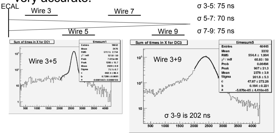
The only explanation is that the width is mainly due to non orthogonal tracks!
