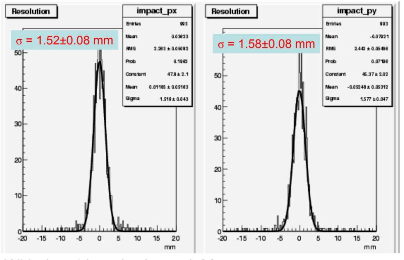
With the old method  $\sigma$  = 1.66 Assuming perfect resolution and including only multiple scattering effects the best resolution is:  $\sigma$  = 0.66
