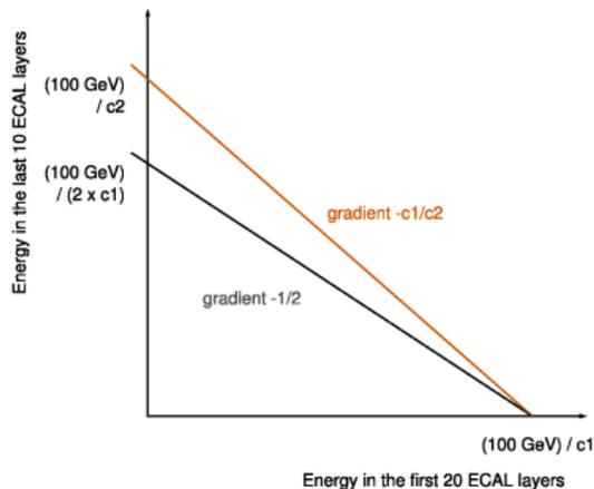
Figure: Correspondance between  $c_1$ s and the ECAL energy plane
