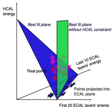
Figure: Fitting a plane in 3-space, rather than a line to 2-space
