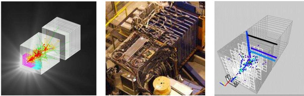
Fig. 1. Simulated pion shower in the CALICE setup with ECAL, AHCAL, and TCMT (left), view of the installation area at the CERN test beam (middle), and a pion event in the on-line display (right).
