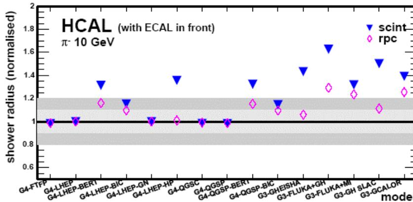
Figure 1.1: Normalized shower radius in a hadron calorimeter as predicted by different hadron shower models.
