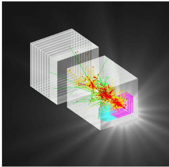
*Figure 3.2 A simulated hadron event in the combined testbeam setup. The ECAL is shown in purple, the AHCAL in white in the centre and the tail catcher in white at the rear.*
