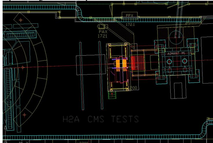
Figure 3.1: Example of integration of the ECAL, AHCAL and tail catcher in beam area H2A.
