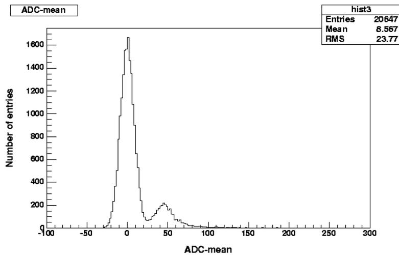
**Figure 2:** Pedestal and cosmic MIP signal on a prototype PCB taken with the VME prototype board.
