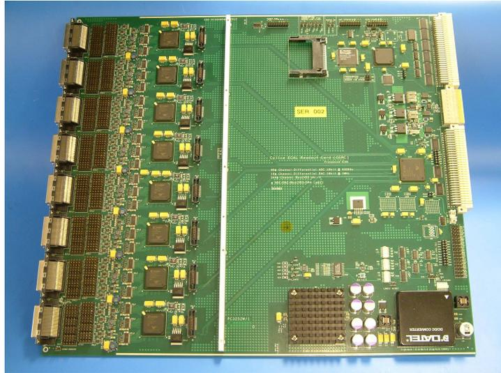
**Figure 1:** Prototype VME readout board.
