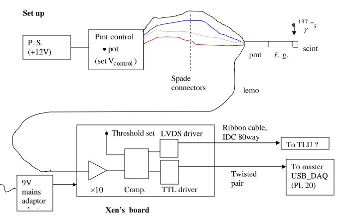
The pmt gain is set by supplying a low voltage (0.9V maximum) via a potentiometer in a control box which is fed by a +12V power supply (IsoTech Lab supply). This control voltage can be monitored from the control box by a DVM. Typically the control voltage is 0.65V.
