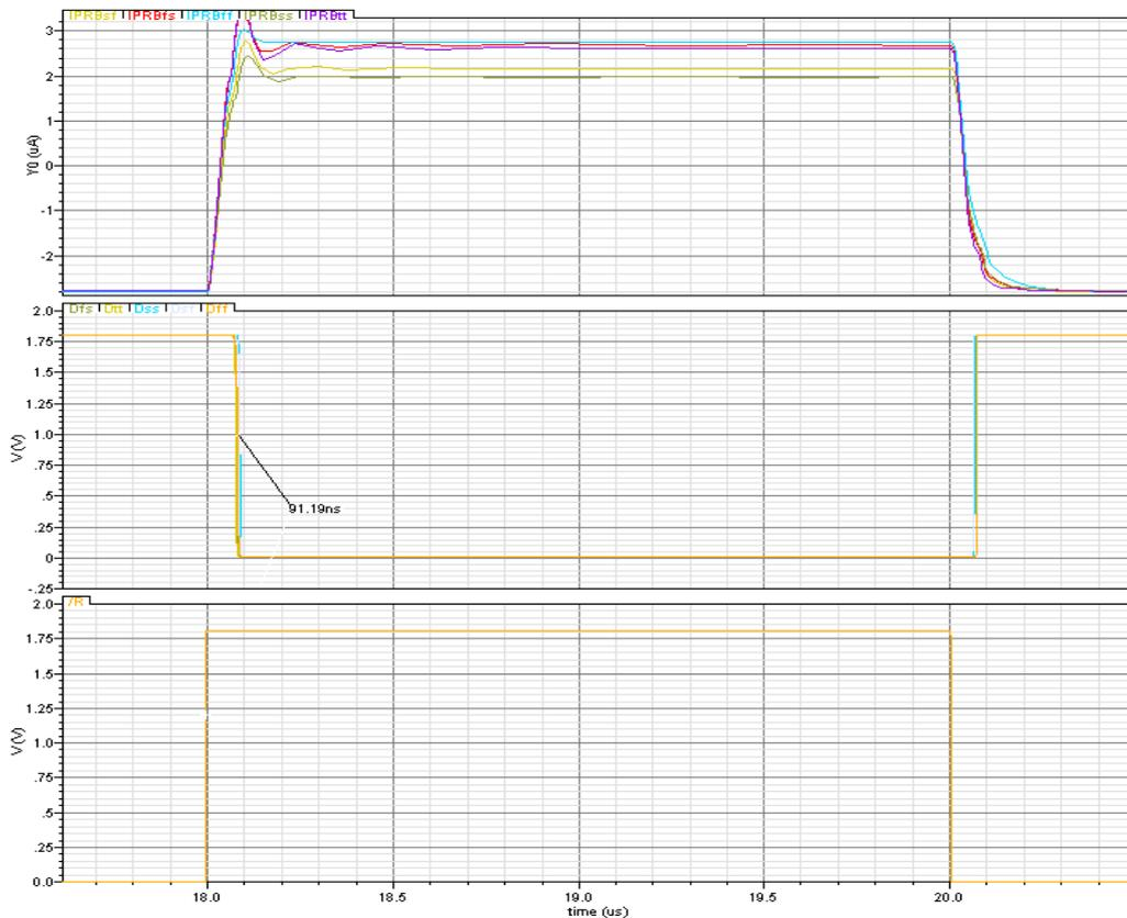
Above: Process corner variations have negligible effect on the operation of this circuit. The bias circuit (which was originally designed for the OPIC project) includes stacked transistors to try to maintain consistent switching performance in different process corners; this seems to be working in this process also, and has not been modified.
