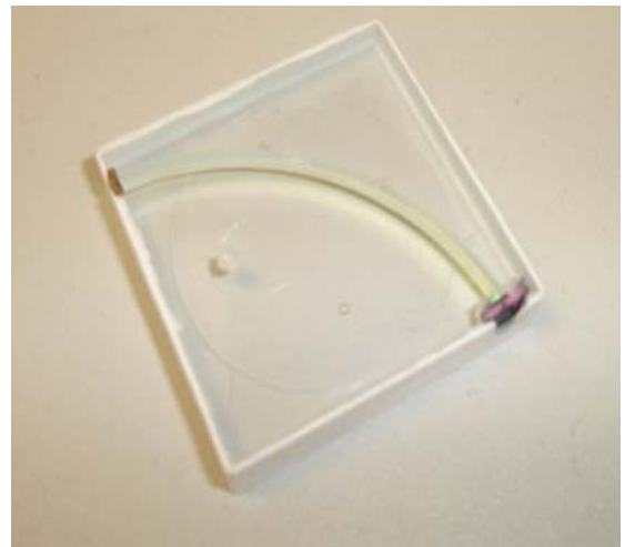
Figure 4-2: Left: SiPM on a support plate. Right: SiPM inserted into a 3x3cm 2 tile.
