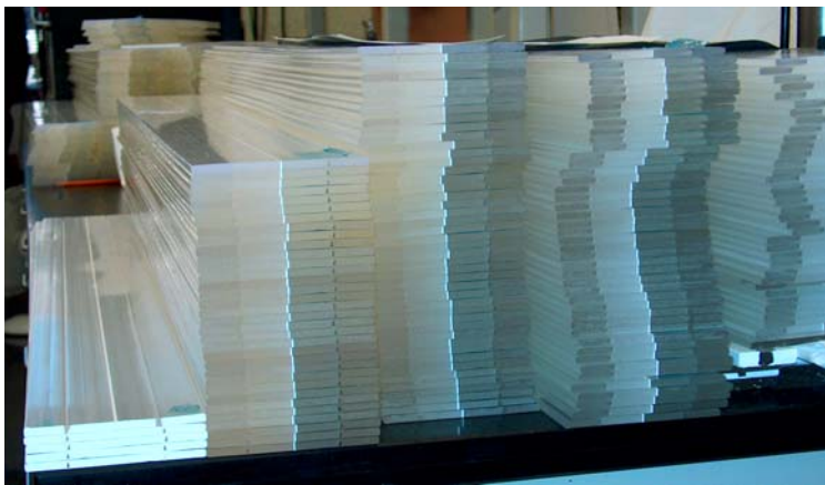
Figure 5-1: Left: Extruded scintillator strips to be used for the TCMT. Right: Normalized response of a set of Kuraray Y11 WLS fibres that will be installed in the TCMT.
