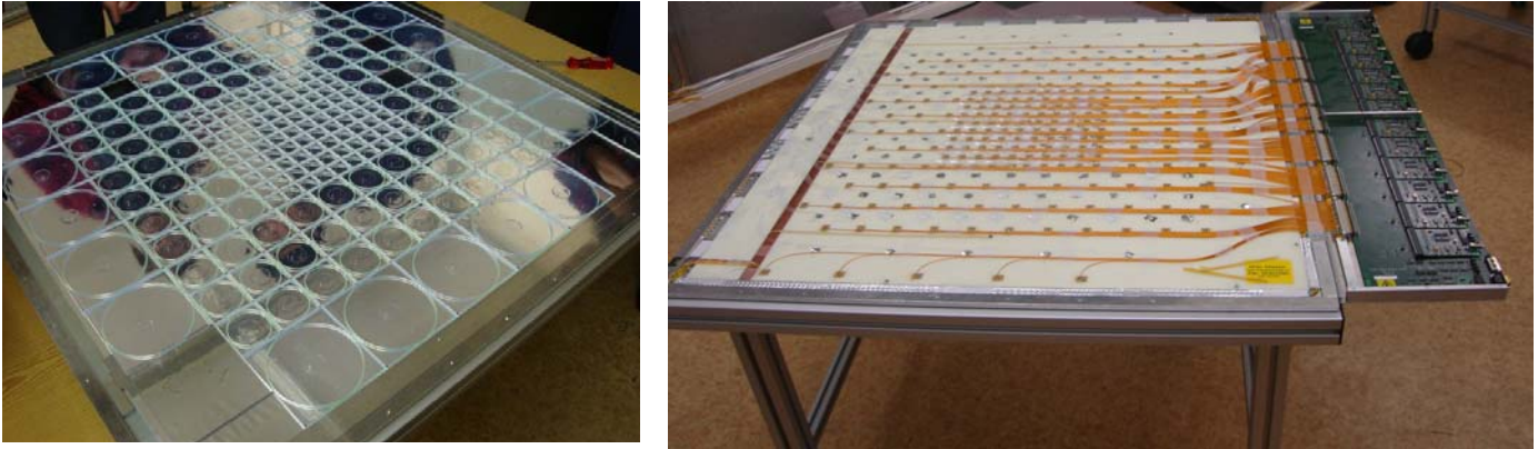
Figure 4-4: Left: Scintillator tile layer. Right: Complete module with front end electronics.
