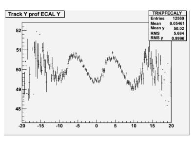
• Correct only for slope; intercept is ECAL alignment = 2.9,50.0
