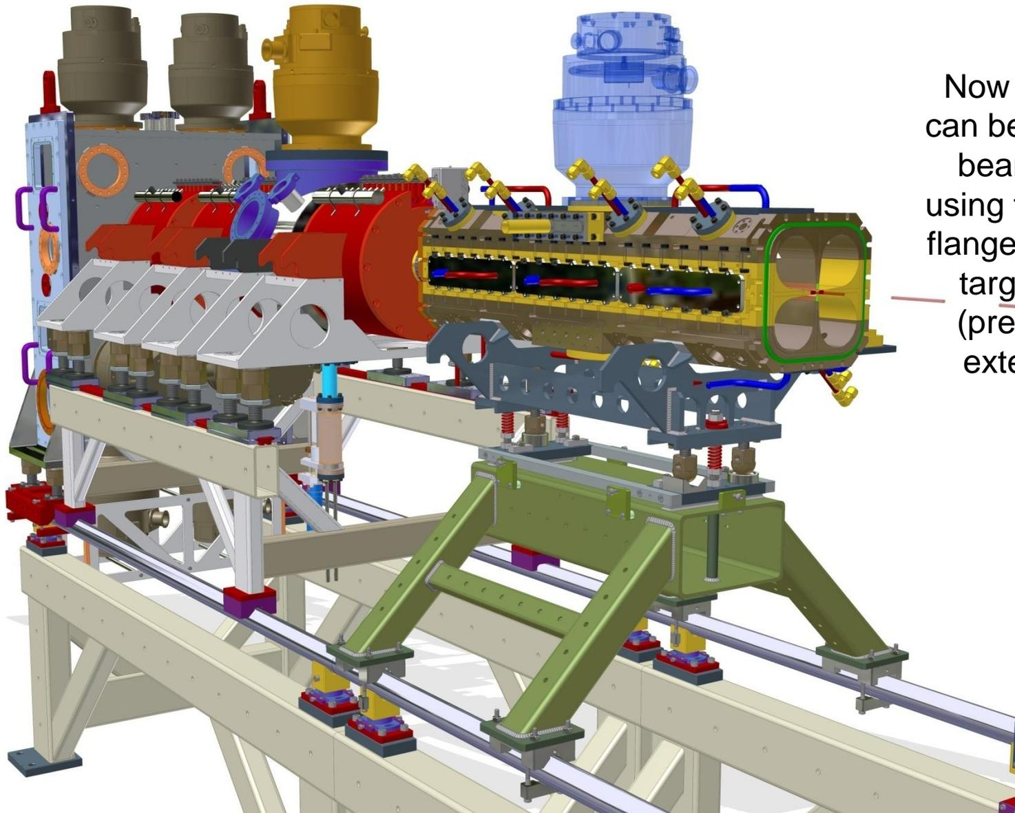
Now the RFQ section can be positioned to the beam axis either by using the alignment end flanges equipped with a target or by using a (previously) defined external reference.
