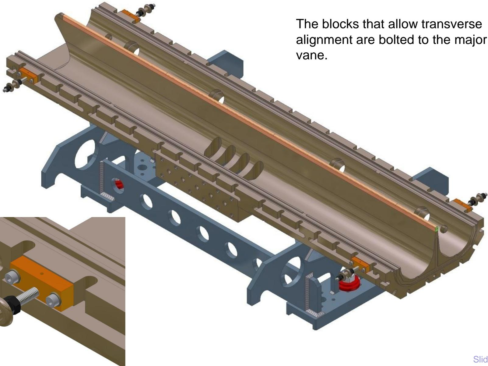
The blocks that allow transverse alignment are bolted to the major vane.
