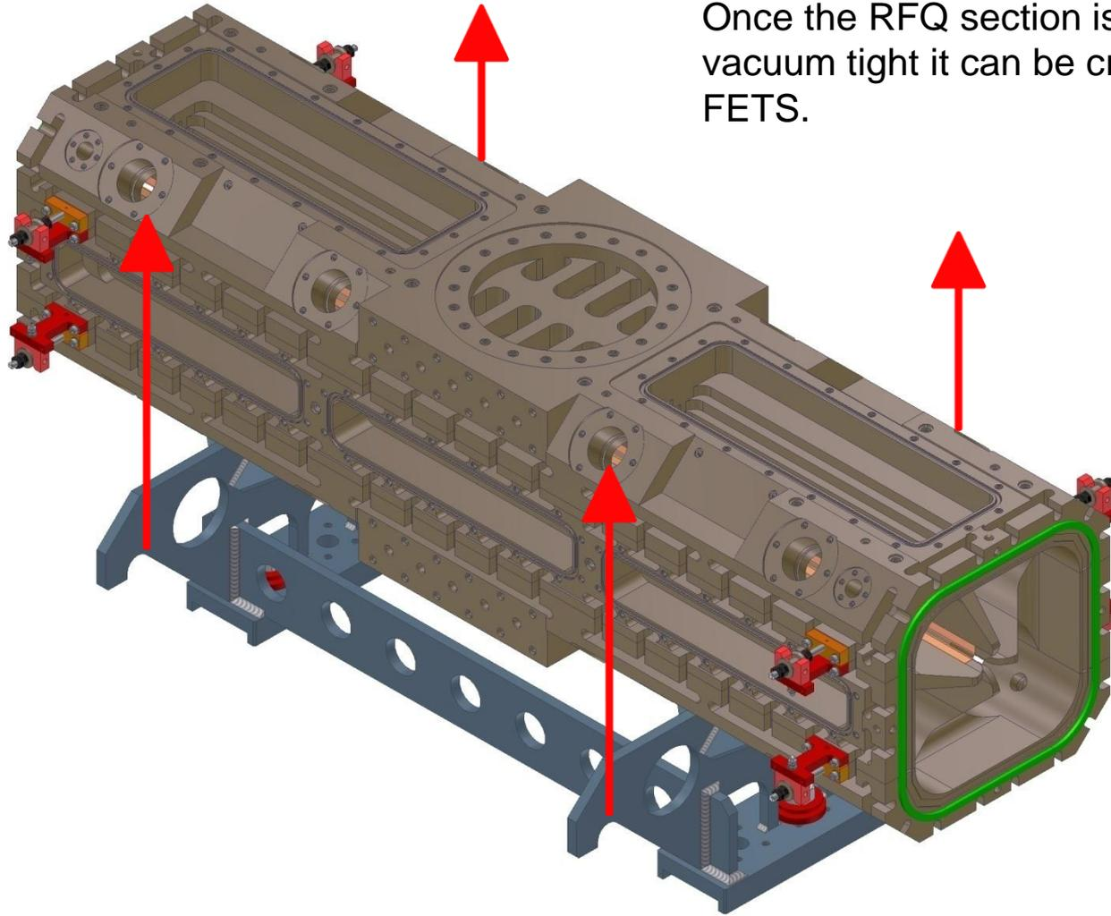
Once the RFQ section is aligned and vacuum tight it can be craned onto the FETS.
