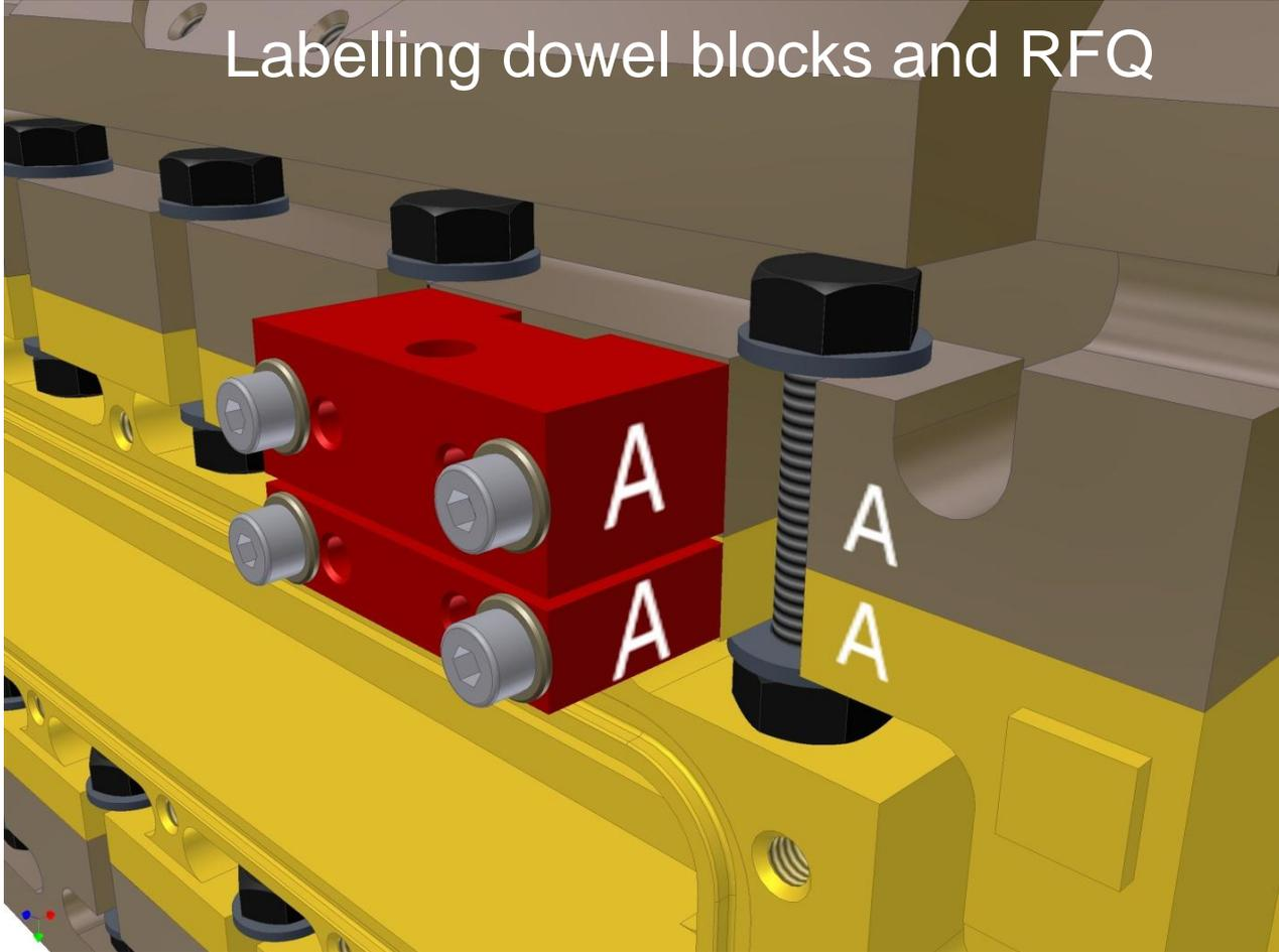
Each dowel block pair now has a unique orientation and position on the RFQ assembly. They may never need to be removed but in case they need to be replaced by the alignment blocks they must be labelled.
