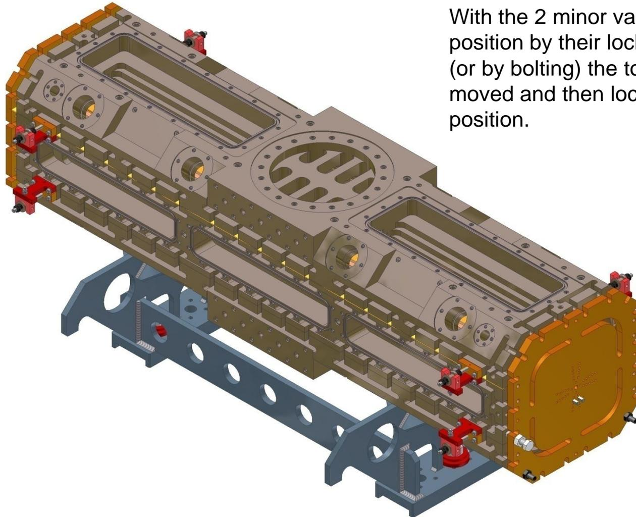
With the 2 minor vanes held in position by their locked adjusters (or by bolting) the top vane can be moved and then locked into position.
