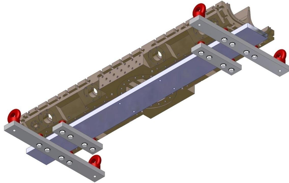
With the protective cage removed the major vane can be lowered into the cradle.
