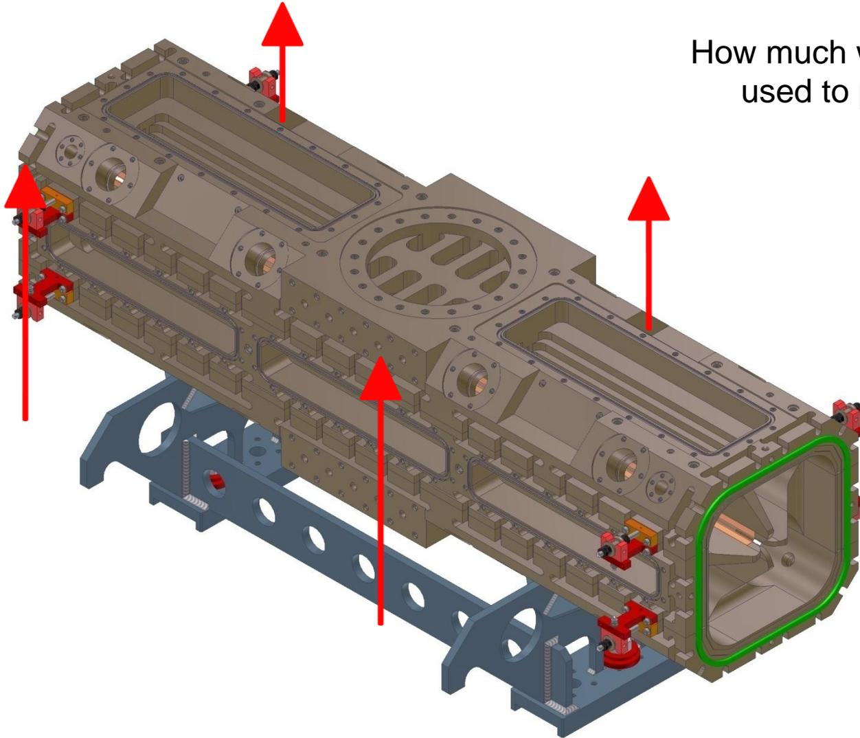
How much will the cradle distort when used to pick up the whole RFQ section?
