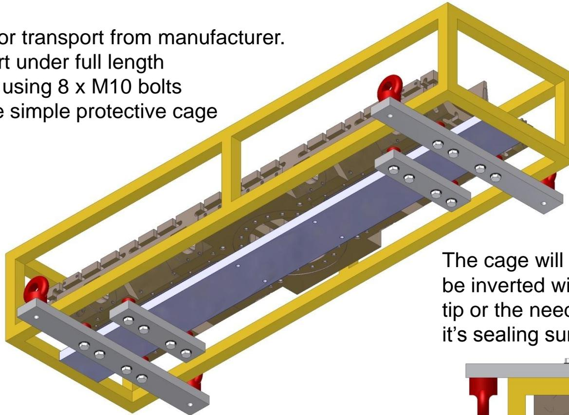
The cage will also enable major vane to be inverted without damage to the vane tip or the need to rest the major vane on it's sealing surfaces.
