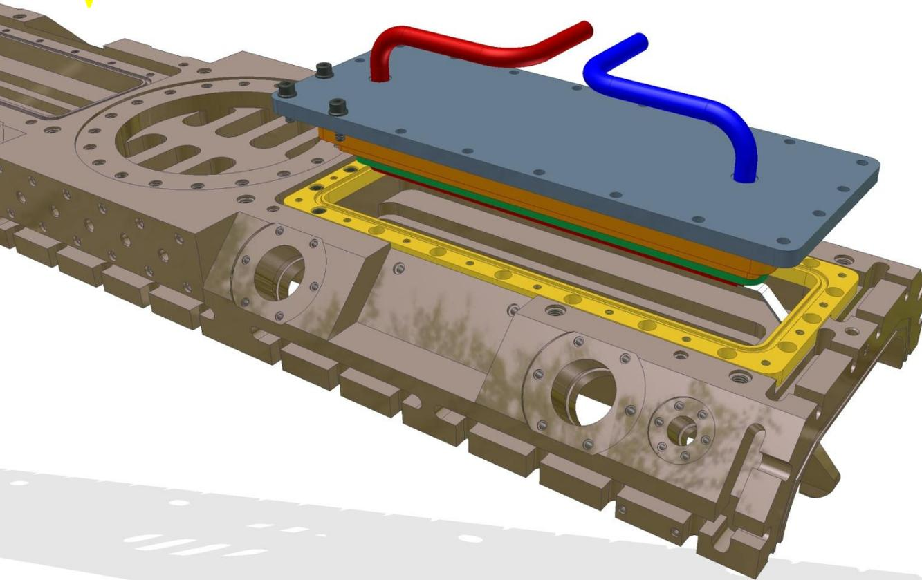
It will be easier to fit the baffles into the lower major vane with it inverted.
