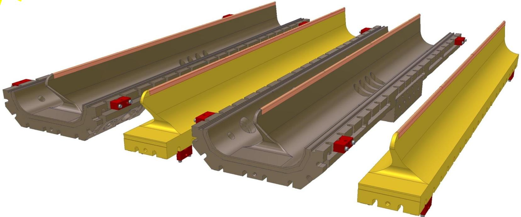
Now the finished pieces of RFQ section 1 can be dismantled leaving the drilled & labelled dowel blocks in position. The new machining of the end faces must now be deburred. This stage can be done either at the manufacturer or at RAL. We are now ready for reassembly with the O ring in place.
