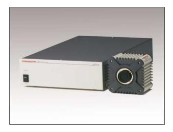
The ORCA-ER is a B/W CCD digital camera using an advanced progressive scan interline CCD chip with high sensitivity in VIS-NIR region offering substantially better noise characteristics at high frame rates. The Peltier cooled hermetic vacuum-sealed head can be cooled to -20°C, reducing dark noise and minimizing thermal drift which makes this camera an ideal choice for demanding scientific and industrial applications.
