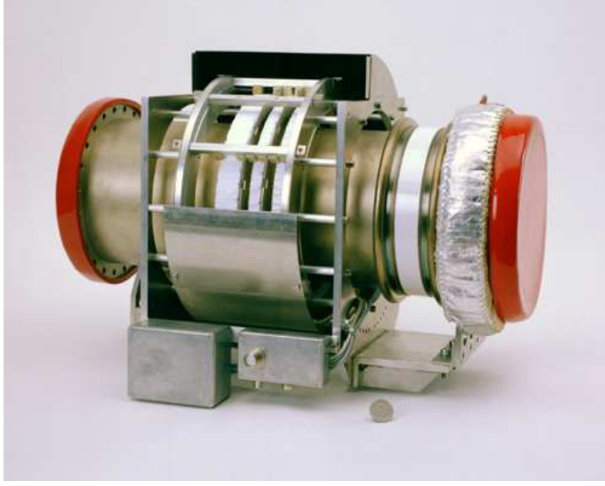
Figure 2.14: The dc-transformer installed at the GSI synchrotron. The left torus is the dc-transformer (two tori mounted closely together), the middle is the ac-transformer used for the feedback of the dc-type and the right one is the ac-transformer for the control of the injection.
