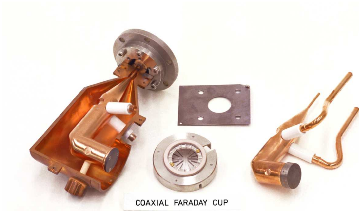
Figure 6.17: Head of a coaxial Faraday cup. The grid for shielding of the advanced field and suppression of secondary electrons is shown in the middle. The collector including the ceramic cooling water feed-through is seen on the right hand side.
