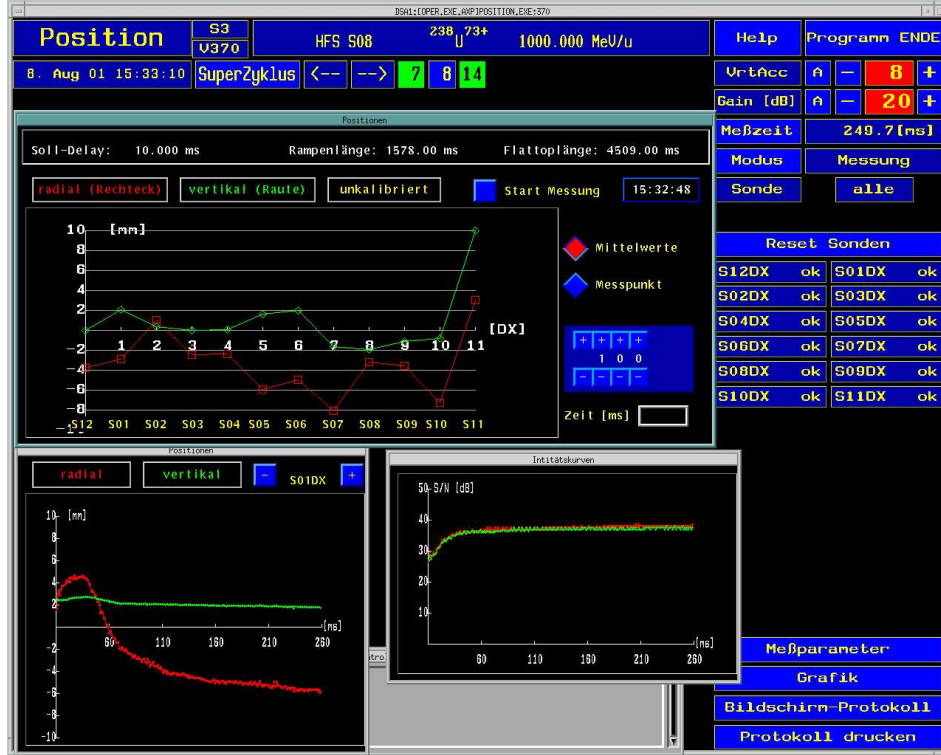
Figure 5.24: Example of a position measurement done at the GSI synchrotron for a partly misaligned beam during the acceleration. The top plot shows the position around the ring at a certain time, the lower left is the position for one pick-up and the lower right is the sum signal power \propto U_{\Sigma}^2 during the ramp for the same single pick-up.
