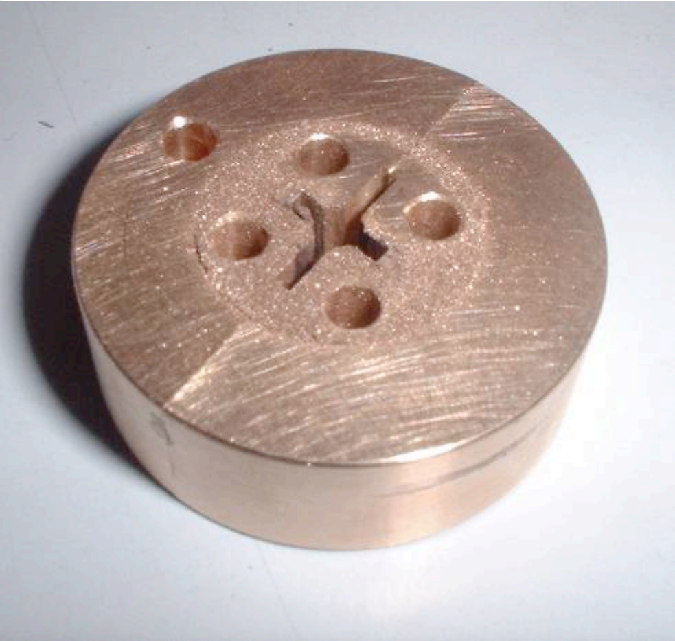
Dust at bottom of housing (after 1.5 M operations)
