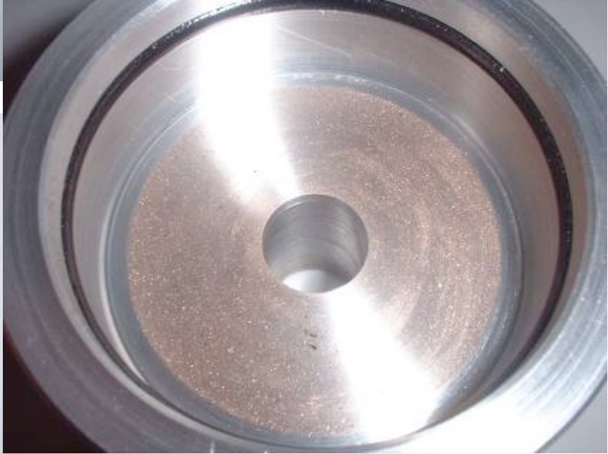
Dust at bottom of housing (after 1.5 M operations)
