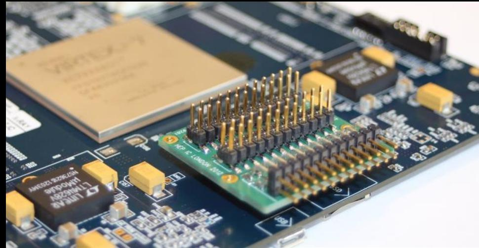
I/O fan-out mezzanine for debugging
