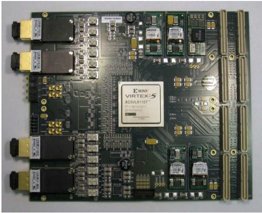
Figure 1: OGTI Card. Xilinx XC5VLX110T FPGA and 4x POP4 optics providing 16 channels at 3.2Gb/s in a dual CMC form factor.
