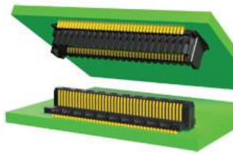
Figure 10 : Samtec SS4-ST4 ultra-fine pitch, high-speed connectors. A single such connector provides 30 differential pairs to/from the FPGA, 3v3, 2v5 and 1v8 supplies and dedicated I2C lines to the microcontroller.
