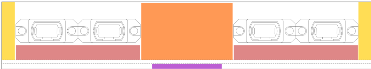
Figure 17 : Front-panel layout of the MP7. Yellow regions indicate \mu TCA infrastructure zones; red regions contains LEDs, etc., the purple region contains the micro-USB connector and microSDHC card connector whilst the orange region indicates the approx. 37mm wide zone available for general-purpose I/O connections. Screw-mount MTP adapters are required to take up any slack in the ribbon cables manufacturing tolerances. Board layout as of 08/02/2012.
