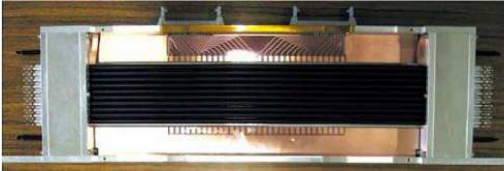
Figure 16.1: Photograph of the prototype electron tracker with seamless straw-tubes.
