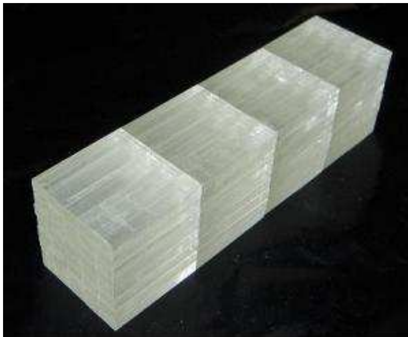
Figure 16.2: Photograph of stacked crystals for a prototype electron calorimeter composed of 160 GSO(Ce) crystals of 4 \times 6 \times 30 mm 3 .
