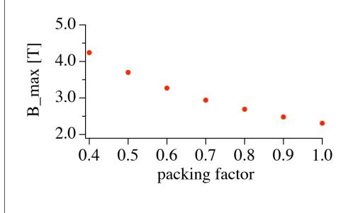
Maximum B fields as a function of magnet packing factor. Average radius and cell tune are fixed at 6.251 m and (0.27, 0.27), respectively. FDF triplet for 0.729 GeV/c beam.
