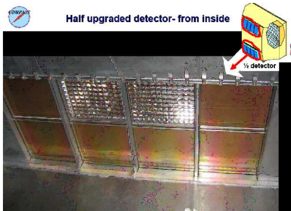
Fig. 5. The COMPASS RICH with central CsI photon detectors replaced by MAPMTs.
