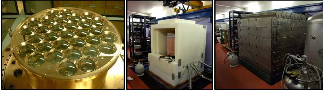
Fig. 1. The PMT array (left), which sits at low temperature inside the LXe vessel; detector located in neutron shield at Boulby (centre); completed lead ‘castle’ (right).
