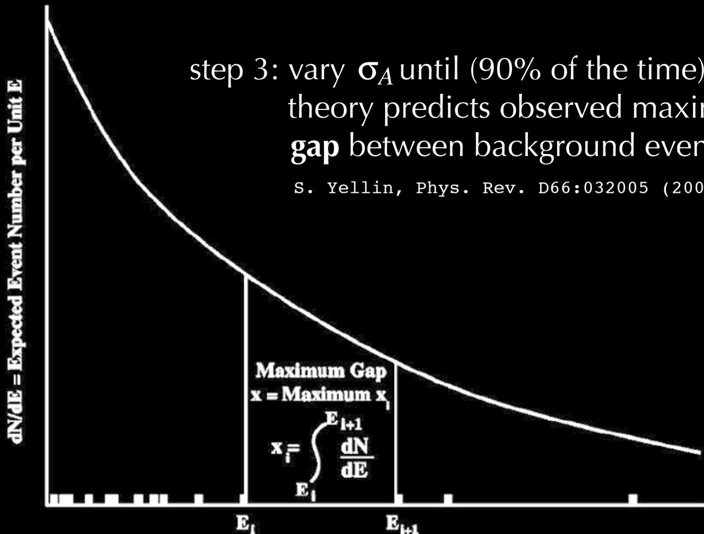
Yellin gap method: a way to make a “zero-background” measurement over a restricted range of an experiment’s acceptance (zero signal too)
