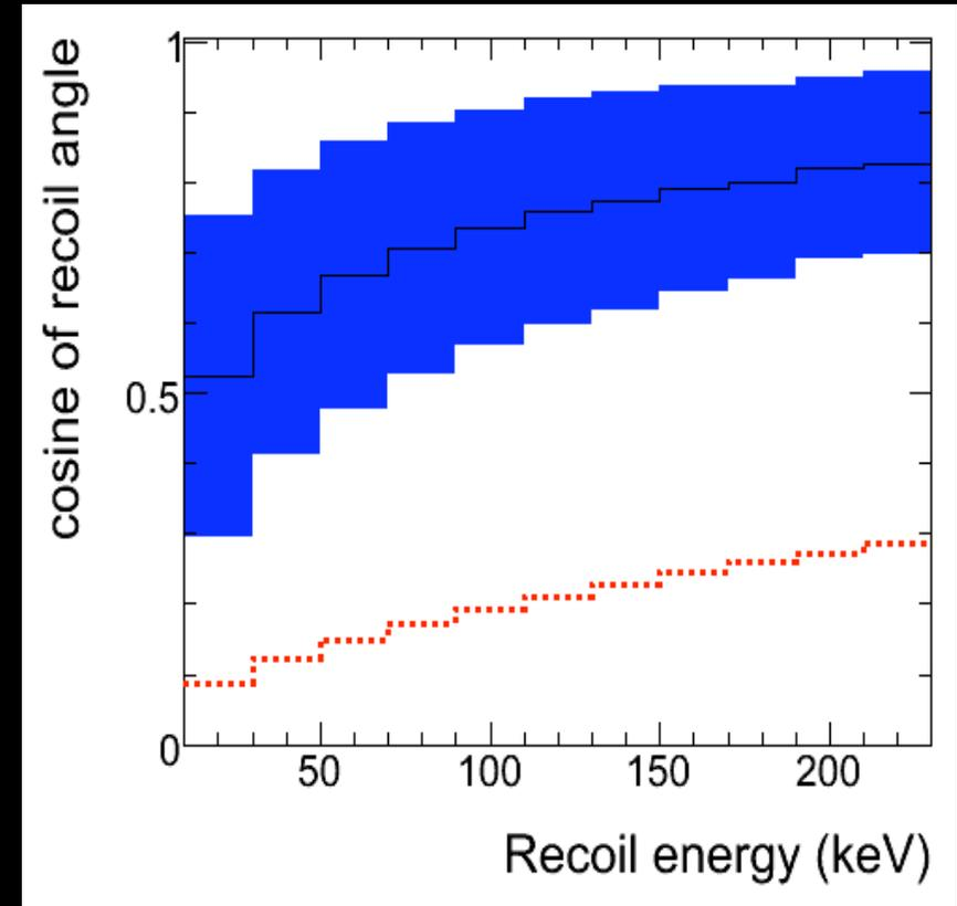
Fluorine recoil momentum better aligned with WIMP direction than neutron recoil
