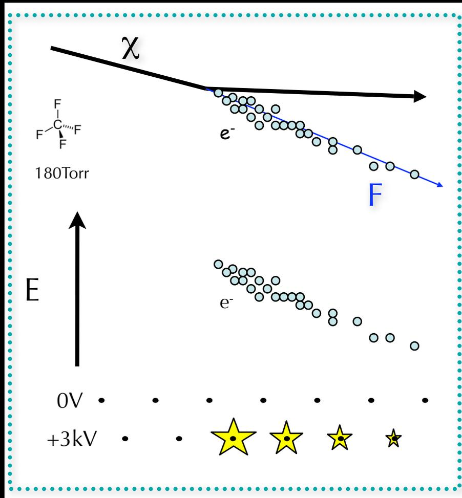
1. primary ionization encodes track direction via  $dE/dx$  profile
