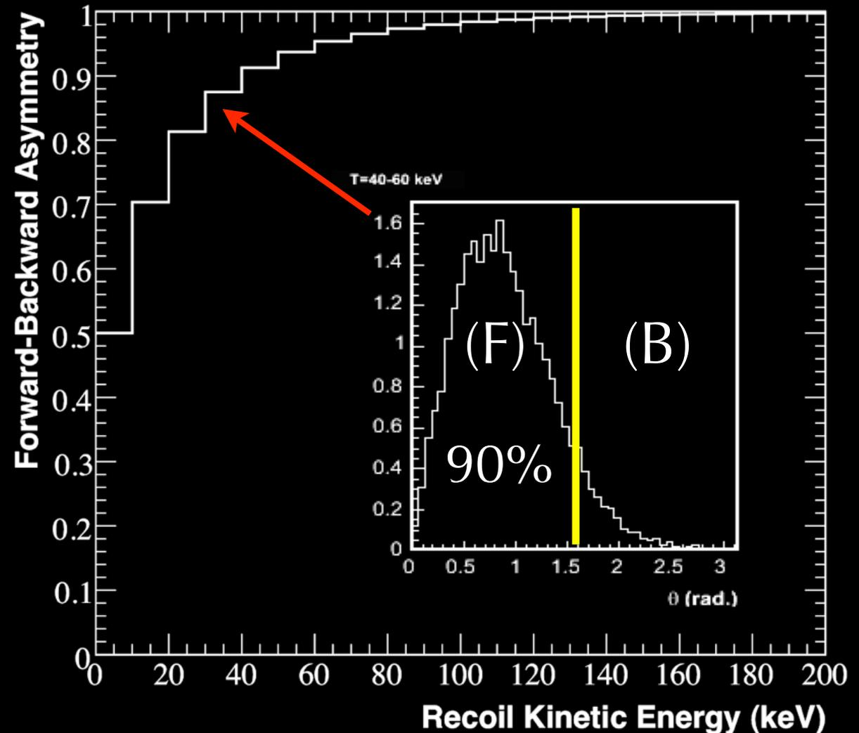
Asymmetry increases with increasing recoil kinetic energy,
