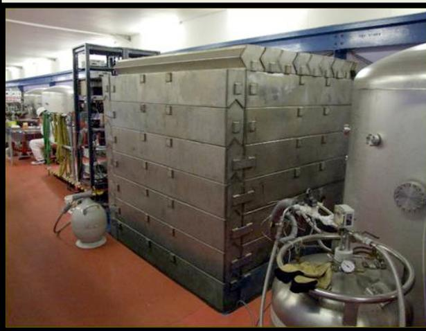
Detector **fully shielded**, with calibration source delivery system and detector levelling mechanism.
