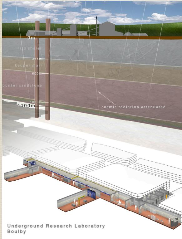
Searching for very rare and small signals requires a very low background. To achieve this the detector is located within a shielding castle, in the Palmer UG lab at Boulby mine.
