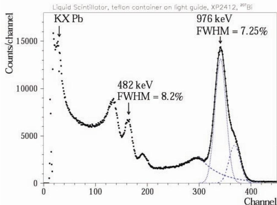
**Energy resolution 4.2% at 3 MeV was measured with 75×75×20 mm LS + light guide + 3" PMT**
