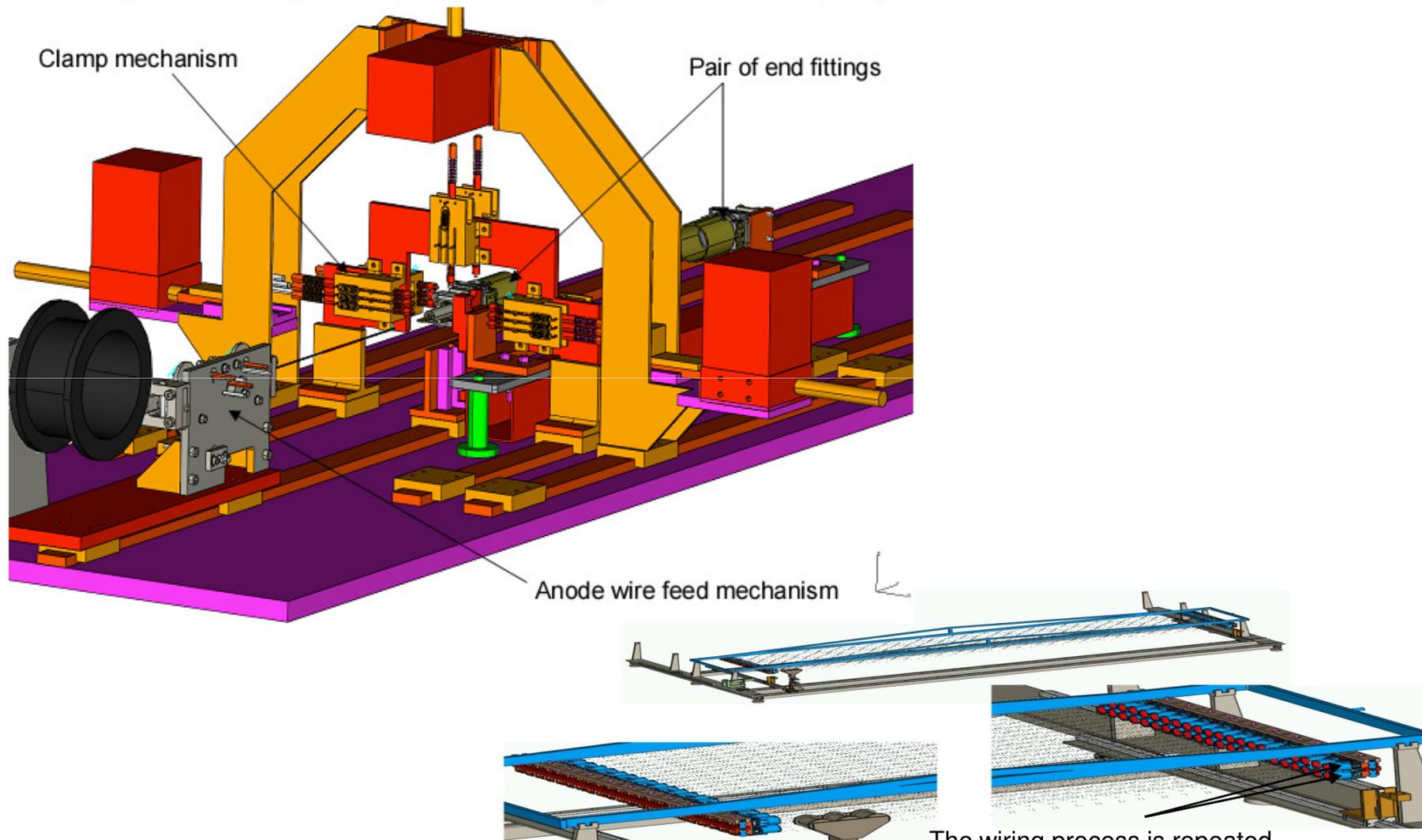
The wiring process is repeated until two complete rows have been produced.
