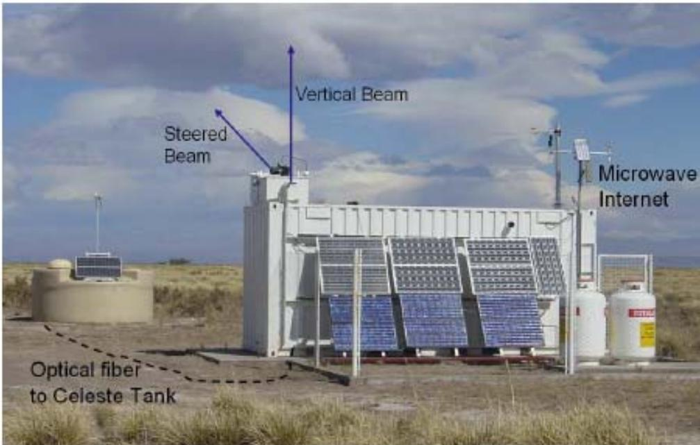
**355 nm, frequency tripled, YAG laser,
