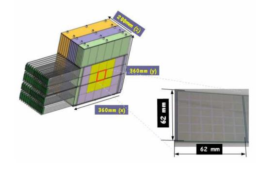
•The prototype ECAL is made in 3 sections of increasing tungsten thickness, and uses 18x18 1cm<sup>2</sup> silicon pads per layer
