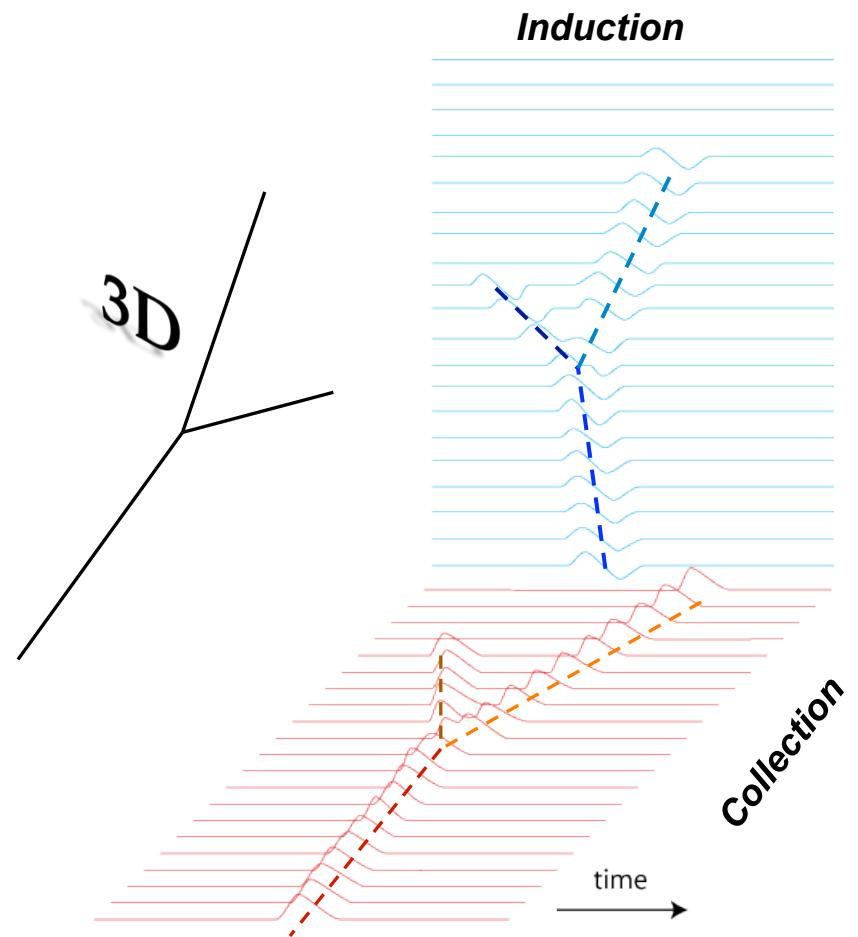
The hits amplitude on the Collection plane, the hit time and the track pitch  $\delta X$  are the fundamental quantities for calorimetry reconstruction
