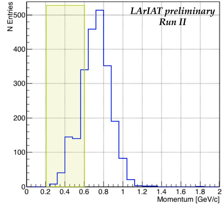
The momentum distribution for kaons in the LArIAT tertiary beamline **overlaps** completely with the momentum spectrum expected for the kaon on a proton decay event.
