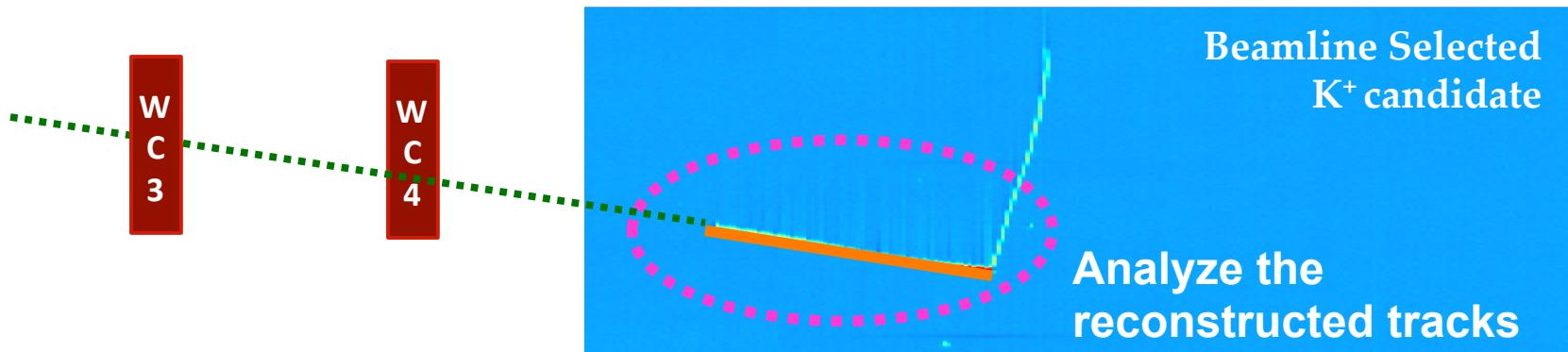
The **K.E.** at **each point** of the TPC track is calculated by subtracting the **track deposited energy** from the K.E. at the TPC front face.
