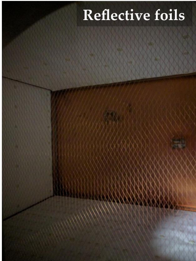
Wavelength shifting (evaporated) **reflector foils** to shift the scintillation light into the visible spectrum
