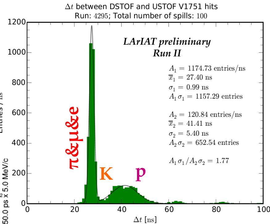
**Particle ID and momentum determination** are performed **before** the particle enters **TPC**!
