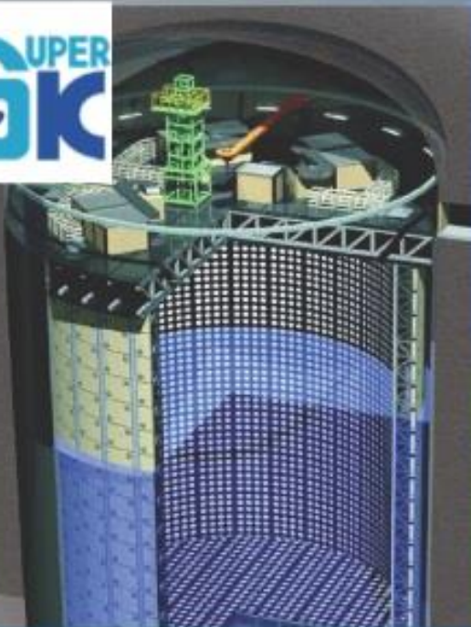
Super-Kamiokande 50 kton water cherenkov detector at 295 km
