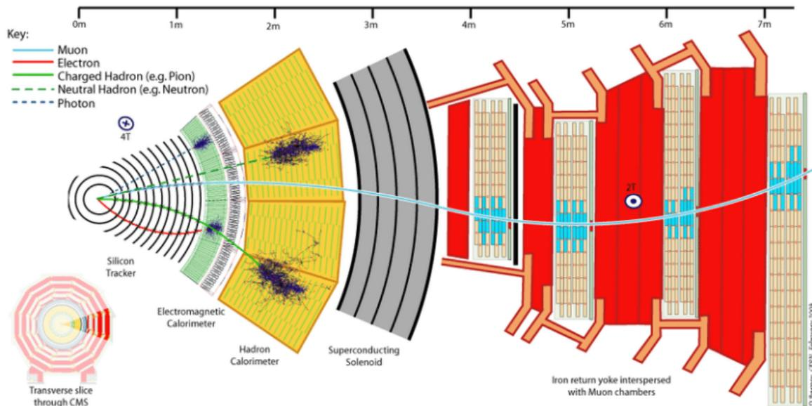
Figure 3: Cross-sectional view of the CMS detector[3].
