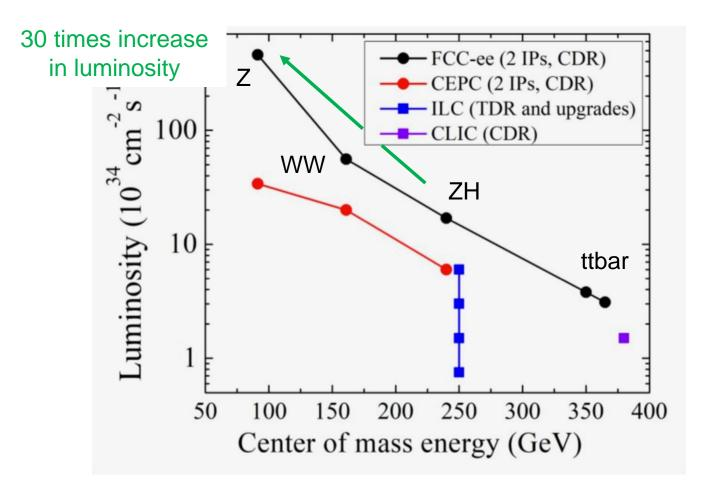
FCC-ee has great capabilities in Higgs physics, but these do not concern us today. L vs E<sub>CM</sub> of a synchrotron means that a very high luminosity Higgs factory (240 GeV) will be an ultra-high luminosity Z factory (91 GeV). Ditto WW production (161 GeV).
