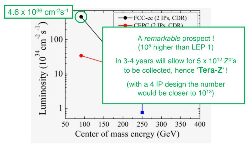
FCC-ee has great capabilities in Higgs physics, but these do not concern us today. L vs  $E_{CM}$  of a synchrotron means that a very high luminosity Higgs factory (240 GeV) will be an ultra-high luminosity Z factory (91 GeV). Ditto WW production (161 GeV).
