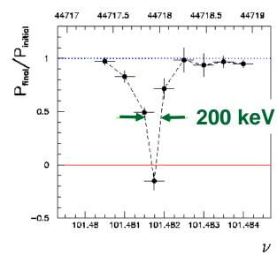
Monitor polarisation with Compton scattering from laser whilst exciting beam with transverse oscillating B field. Find frequency at which depol<sup>n</sup> occurs.
