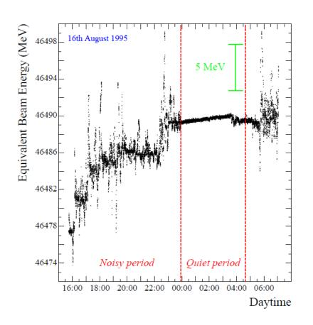
Found to be due to magnets being 'tickled' by current on beam pipe from passing trains.
