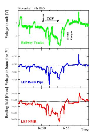
Found to be due to magnets being 'tickled' by current on beam pipe from passing trains.
