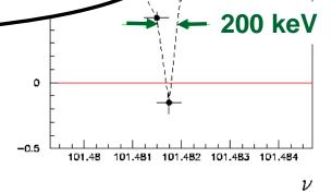
Monitor polarisation with Compton scattering from laser whilst exciting beam with transverse oscillating B field. Find frequency at which depol<sup>n</sup> occurs.
