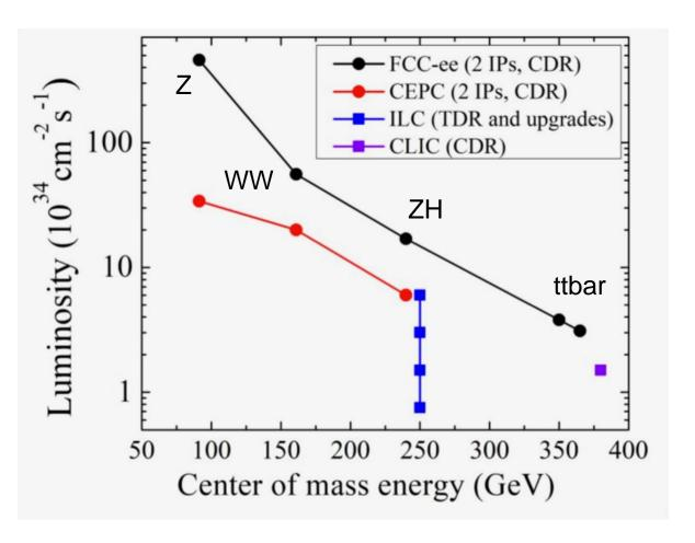
FCC-ee has great capabilities in Higgs physics, but these do not concern us today. L vs  $E_{CM}$  of a synchrotron means that a very high luminosity Higgs factory (240 GeV) will be an ultra-high luminosity Z factory (91 GeV). Ditto WW production (161 GeV).
