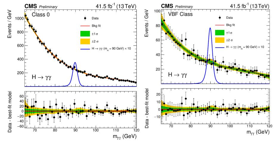
Choice of background function is discrete parameter in lh fit to data, systematic error associated with each possible choice (discrete profiling or 'envelope' method)
