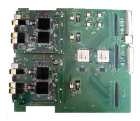
**Figure 2.11:** The GCT wheel card. From left to right, are two dual-PMC sites (with leaf card fitted but no interconnecting ribbon cables), two Xilinx Virtex-4 FPGAs, three high-speed connectors and VME64x connectors (power only). At the top and bottom of the card are two cutouts through which the ribbon cables pass.
