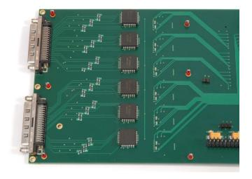
**Figure 3.7:** The RCT Emulator card. The card is mounted on an IDAQ card by means of 0.1 inch pitch header and acts as a logic-level translator. The central integrated circuits are six-channel TTL-ECL converters driven by the FPGA on the IDAQ. The ECL output is subjected to a -5 V bias and output on two VHDCI SCSI connectors.
