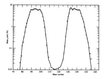
Note the nuclei tend to be unequal, despite the energy release being maximum for an equal division.
