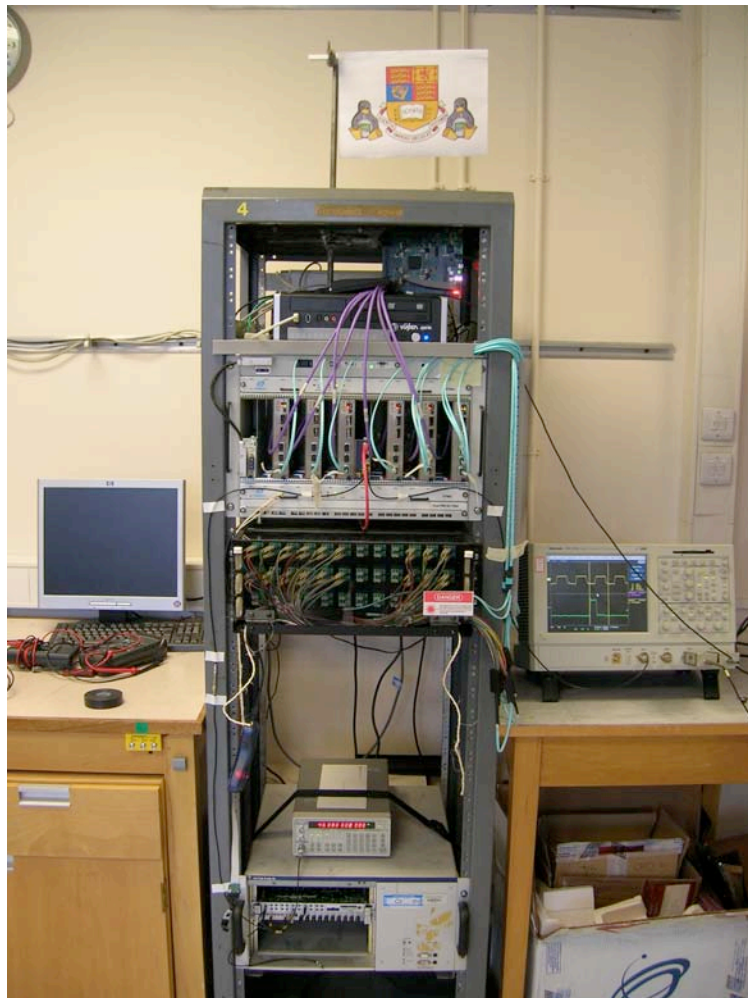
Fig. 5.1. MINI-T5-R2 cards, designed at Imperial College and manufactured by eXception PCB Ltd (Tewkesbury, UK) and Cemgraft (Newbury, UK) undergoing system tests at Imperial College.
