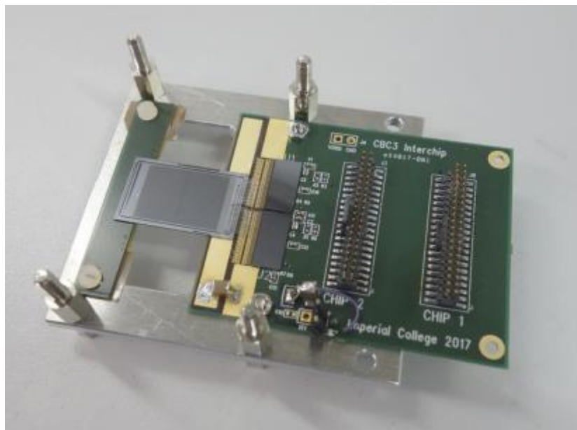
Figure 4.2. A single sensor 2CBC3 module built from a PCB designed at Imperial, with a small sensor attached and wire-bonded. This version includes some of the inter-chip communication signals and will allow this feature to be tested for the first time.
