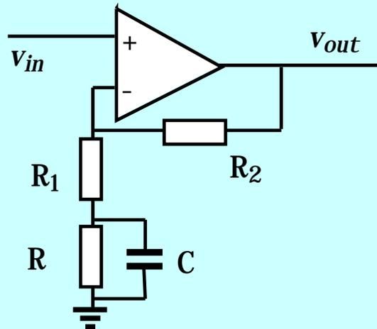
differentiator/high pass filter with gain & inversion
