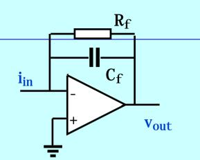
$\begin{array}{ll} \mbox{step replaced by decay with $\sim$ exp(-t/R_fC_f)$ is long because $R_f$ is large (noise)$ easiest way to limit pulse pileup - differentiate$ ie add high pass filter$ \\ \end{array}$
