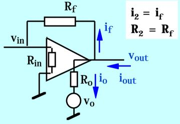
$$\begin{split} Z_{out} &= v_{out} / i_{out} = R_o \, (R_2 + R_{in}) / [Ro + R_2 + R_{in}(A + 1)] \\ R_o / (A + 1) \\ since \ R_{in} >> R_2, \ R_o \end{split}$$
